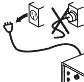
Disconnect electrical power before performing any maintenance.
