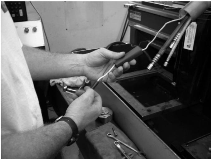
7. Fold the excess pilot arc wire, slide the heat shrink over the folded wire, and apply heat. The loose wire can also be pulled back into the ignition console. Any excess wire in the ignition console must be secured with heat shrink or tape.
