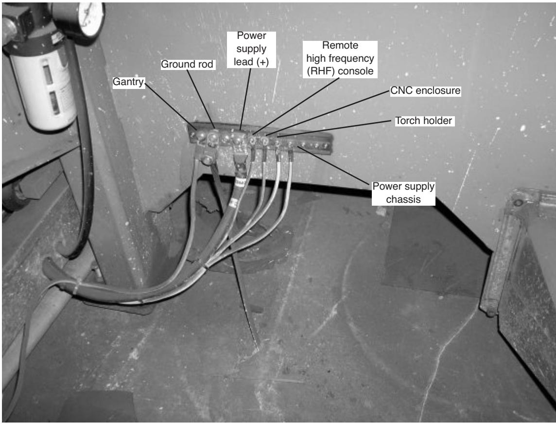
Example of a good cutting table ground bus. The picture above shows the connection from the gantry ground bus, the connection from the ground rod, the power supply positive lead, the RHF console, the CNC enclosure, the torch holder, and the power supply chassis.
