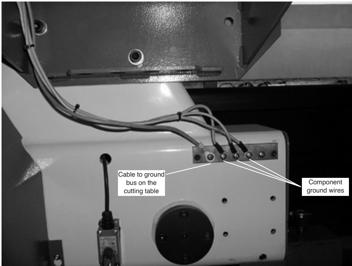
Example of a good gantry ground bus. It is bolted to the gantry, close to the motor. All of the individual ground wires from the components mounted on the gantry go to the bus except those from the RHF module and the torch holder. A single heavy cable then goes from the gantry ground bus to the ground bus bolted to the table.
