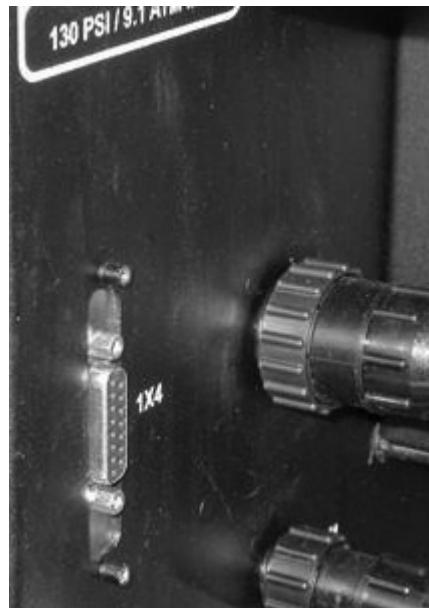
11. Route the cable from the power supply to the Edge Ti and connect the cable to the plasma interface connector.
