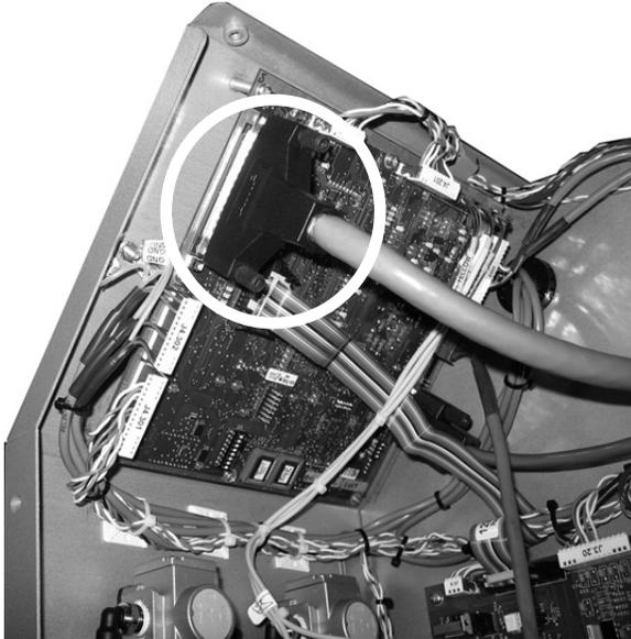
DB-37 connection on the control board
