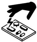
Static electricity can cause damage to printed circuit boards (PCBs). Use correct precautions when you touch PCBs.
