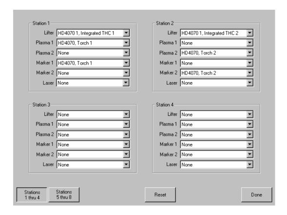
In the previous example, you can see that the Cutting and Marking with the HD4070<sup>®</sup> Integrated Torch 1 is limited to Plasma Process 1 / Maker Process 1 on Station 1. Additionally, the Cutting and Marking with HD4070<sup>®</sup> Integrated Torch 2 is limited to Plasma Process 2 / Maker Process 2 on Station 2. These stations may be configured to Cut or Mark or both. A second multi-dropped HD4070 may be also be assigned on stations 3 & 4.
