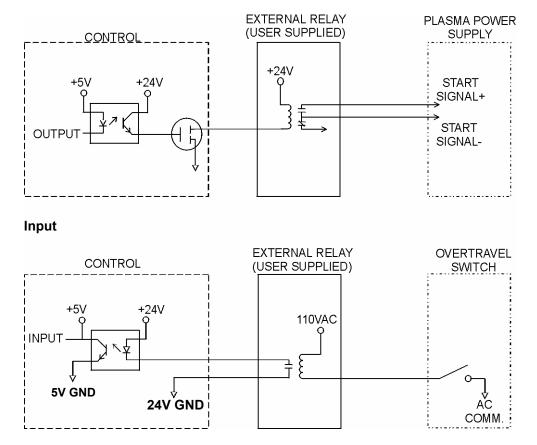
**Single Ended I/O Pinout** The Single Ended I/O offers 12 outputs which are rated at 24VDC for up to 1-amp loads and 12 inputs rated for 24VDC.
