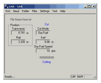
The following is a brief description of the available setup parameters for the Phoenix Link. Simply left click with the computer mouse on the selected feature in the drop down box to select, enable or execute that feature.
