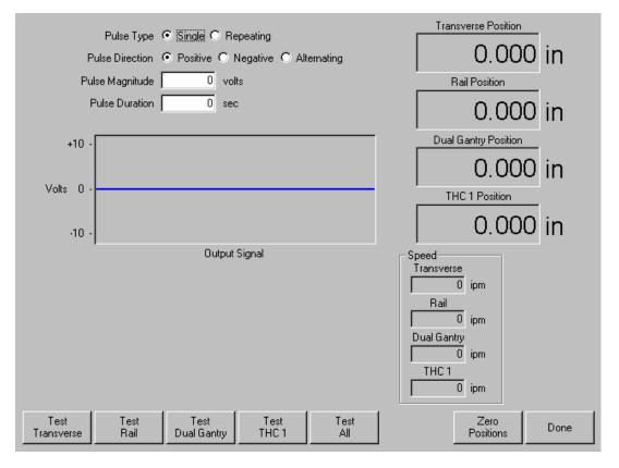
The Voyager II<sup>™</sup> control has the ability to control up to six axes of motion. When entering the Drives & Motors Diagnostic screen, the user will prompted to select which group of axes will be available for testing.
