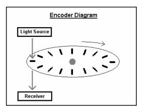
As there is a direct relationship between the rotation of the motor shaft, the Encoder Pulses and the distance of motion traveled (when the motor shaft turns) the control is able to calculate distance by counting the encoder pulses received, thus closing the Position loop. So this relationship shown as a simplified formula would be:
