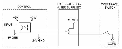
**Single Ended I/O Pinout** The Single Ended I/O offers 32 outputs which are rated at 24VDC for up to 1-amp loads and 32 inputs rated for 24VDC as standard
