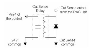
Input tied to Cut Sense Relay
