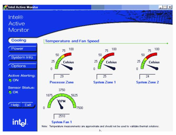
The INTEL<sup>®</sup> Active Monitor allows the user to view Cooling, Power and System information. Additionally, this allows active alerts to set and posted on screen during operation.
