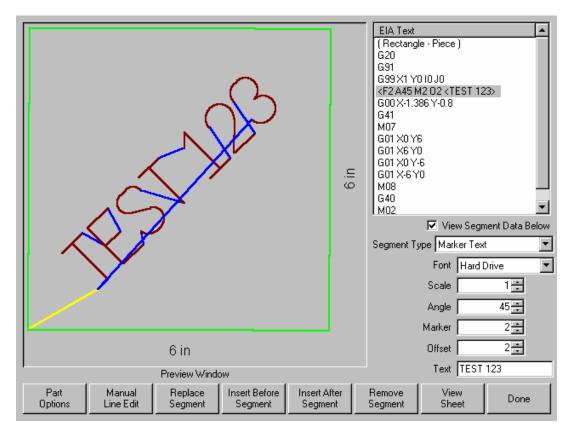
To improve the ease of use for the part program designer and control operator, the Marker Font Generator feature will always insert a traverse segment to return to the original start point at the beginning of the marking text.
