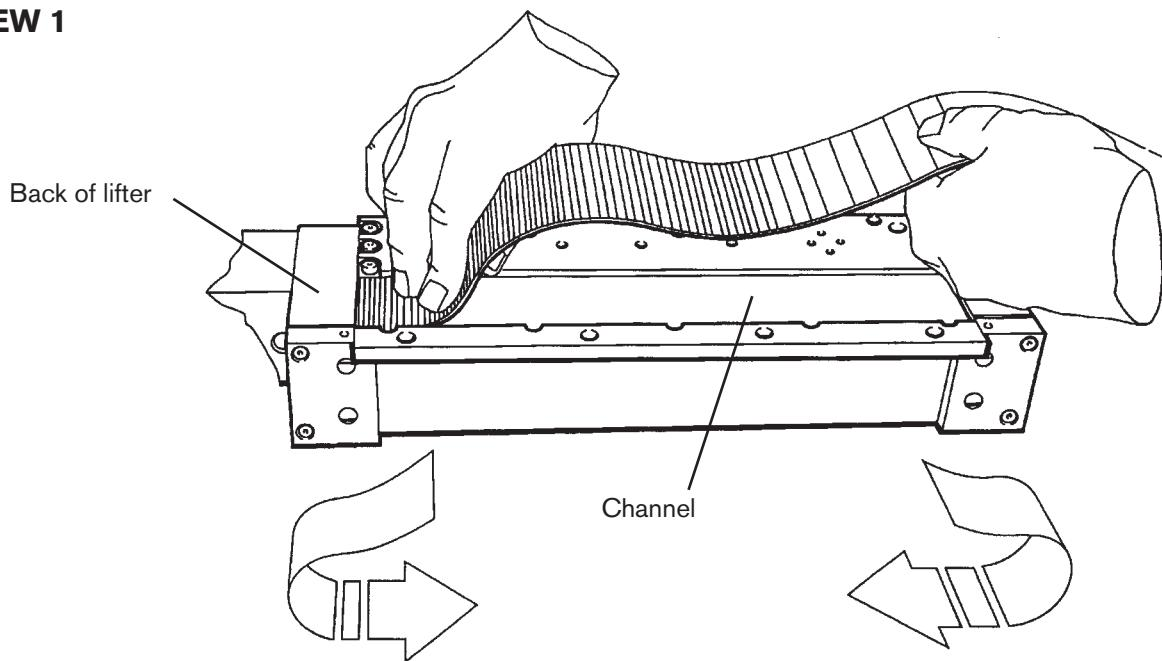
**Figure 5-2 Sealing band – install (1 of 2)**
