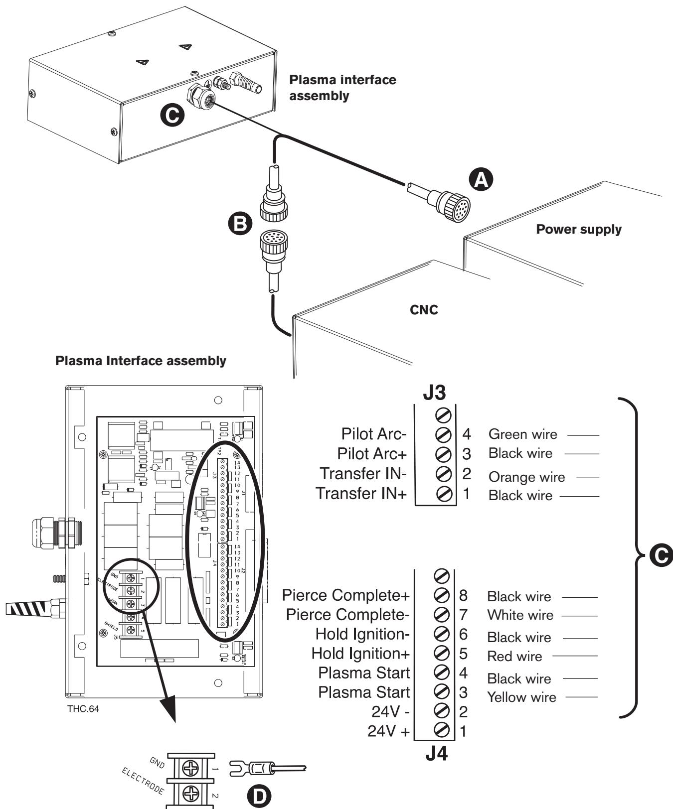
Figure 3a-2 HD3070 Power supply interface cable connections
