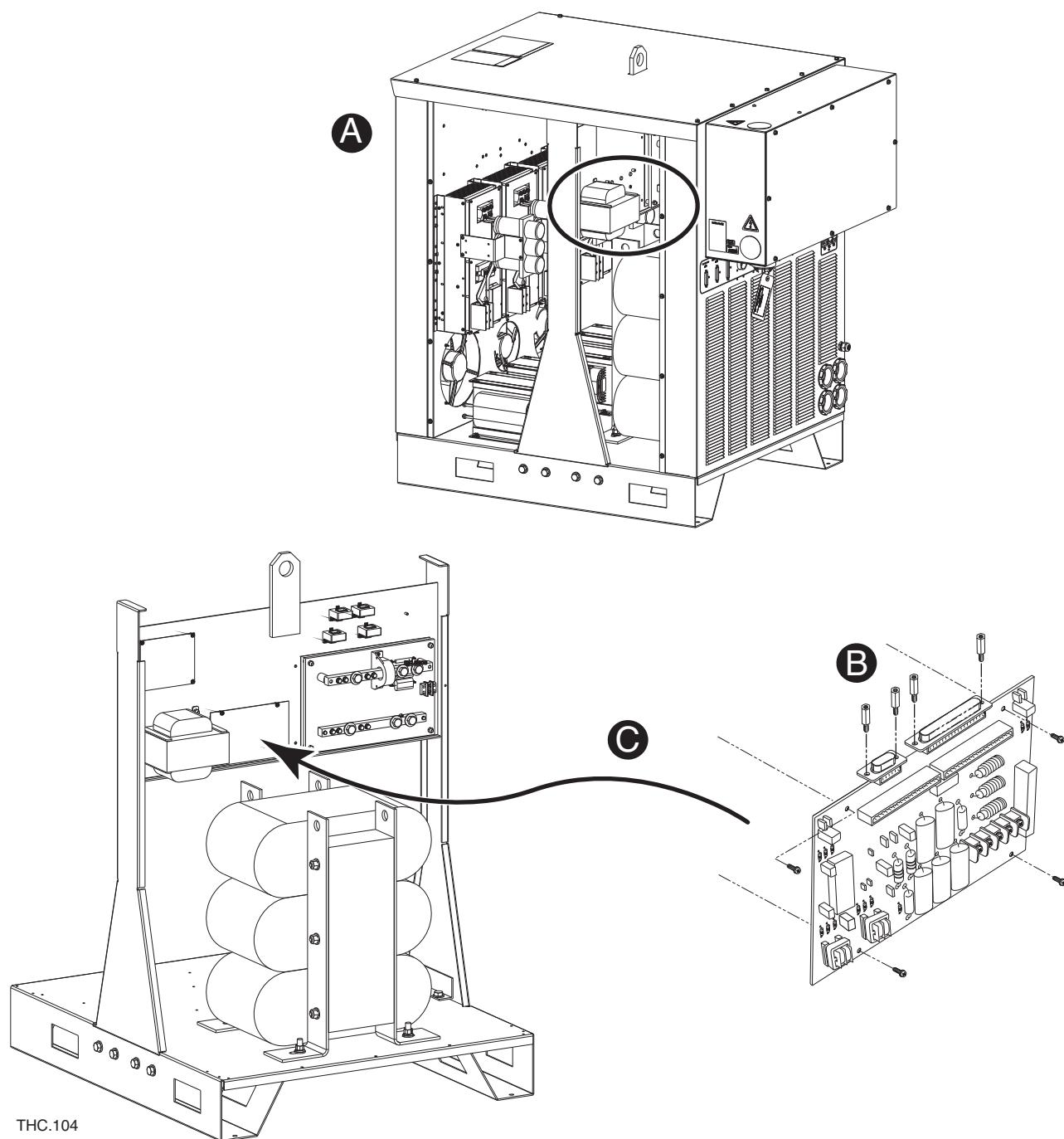
**Figure 3h-2** Install the plasma interface PC board
