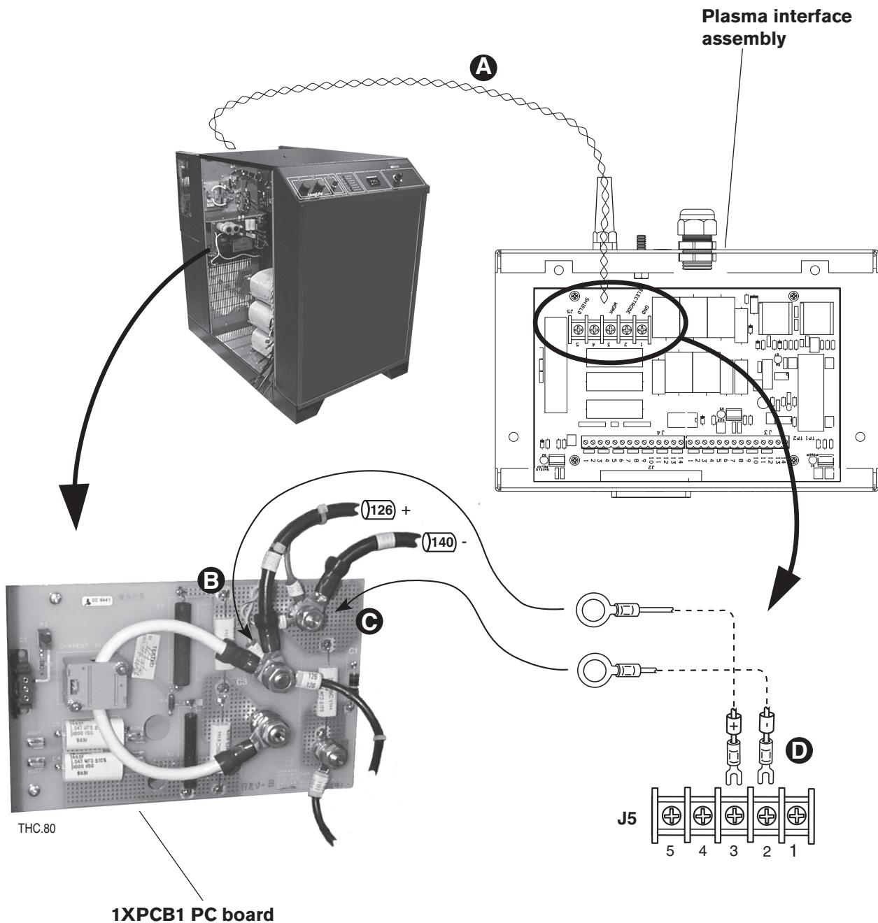
Figure 3a-1 HD3070 electrode and work lead arc voltage wires connection
