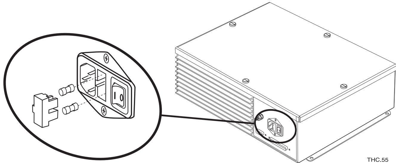
**Figure 5-4 AC power and fuses****Table 5-2 AC power and fuses**
