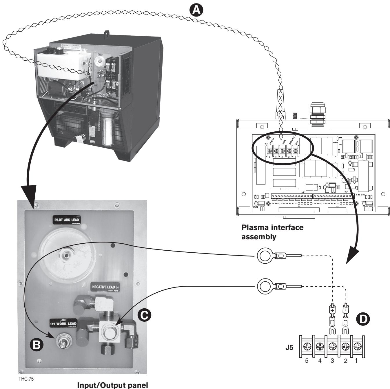
Figure 3f-1 MAX200 electrode and work lead arc voltage wire connections
