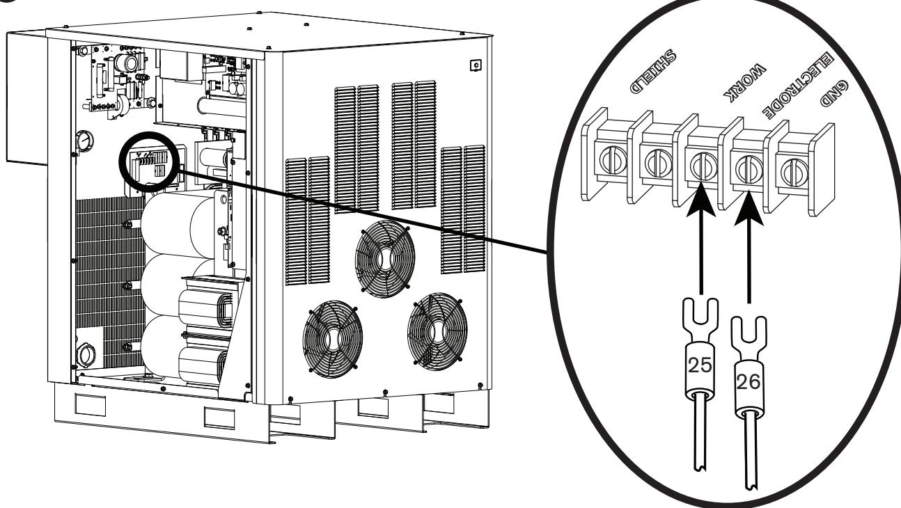
Figure 3i-12 Plasma interface PC board connection
