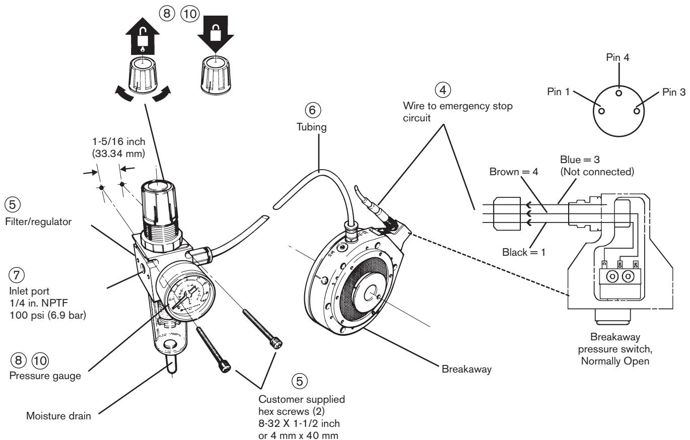
**Figure 3-5 X-Y lifter assembly optional torch breakaway kit mounting details**
