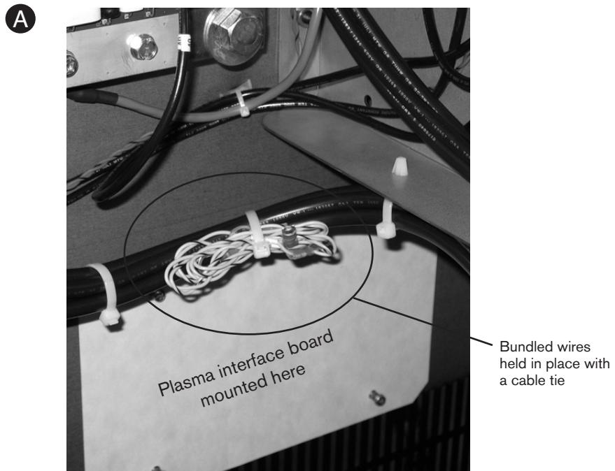
**Figure 3i-11 Plasma interface wire location**
