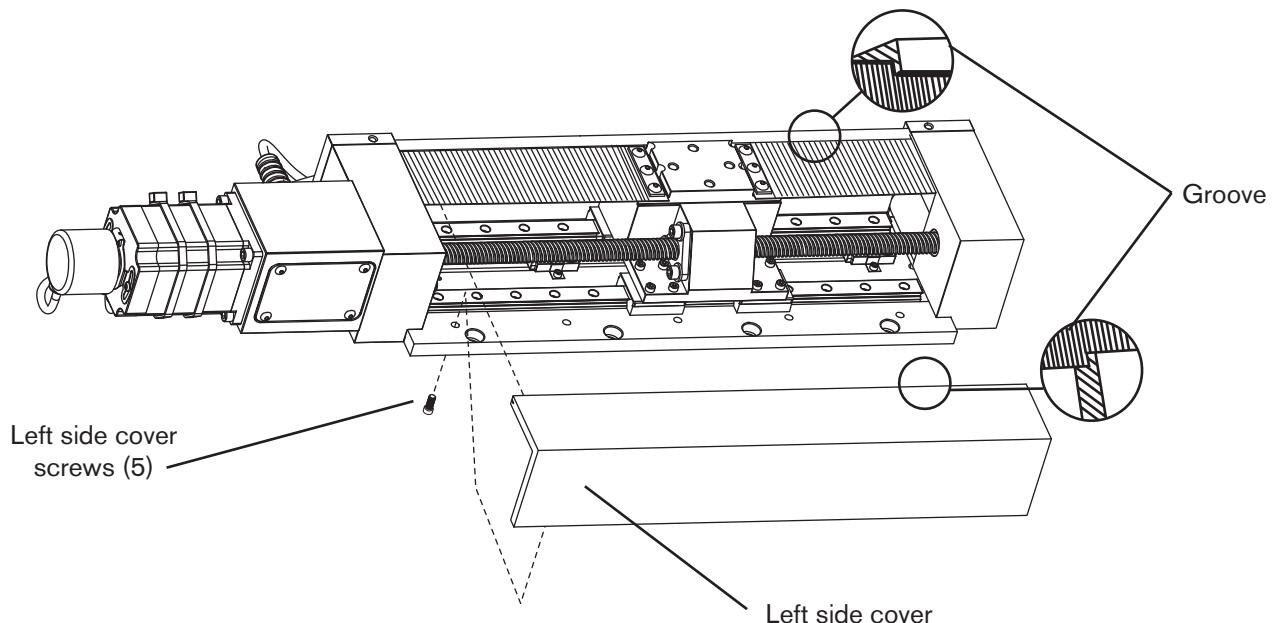
Figure 5-2 Sealing band – install (2 of 2)
