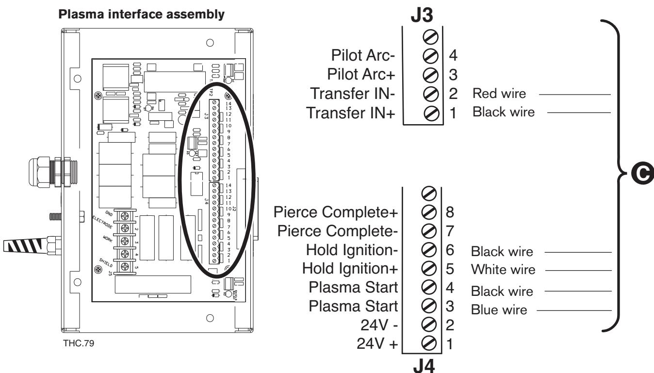
Figure 3d-2 HT4001 power supply interface cable connections
