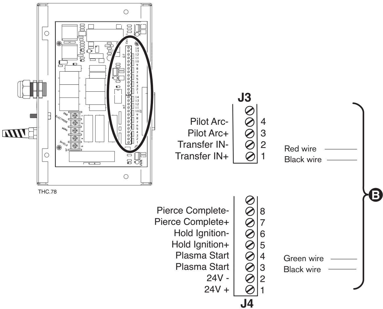
Figure 3g-3 Powermax power supply interface cable connections
