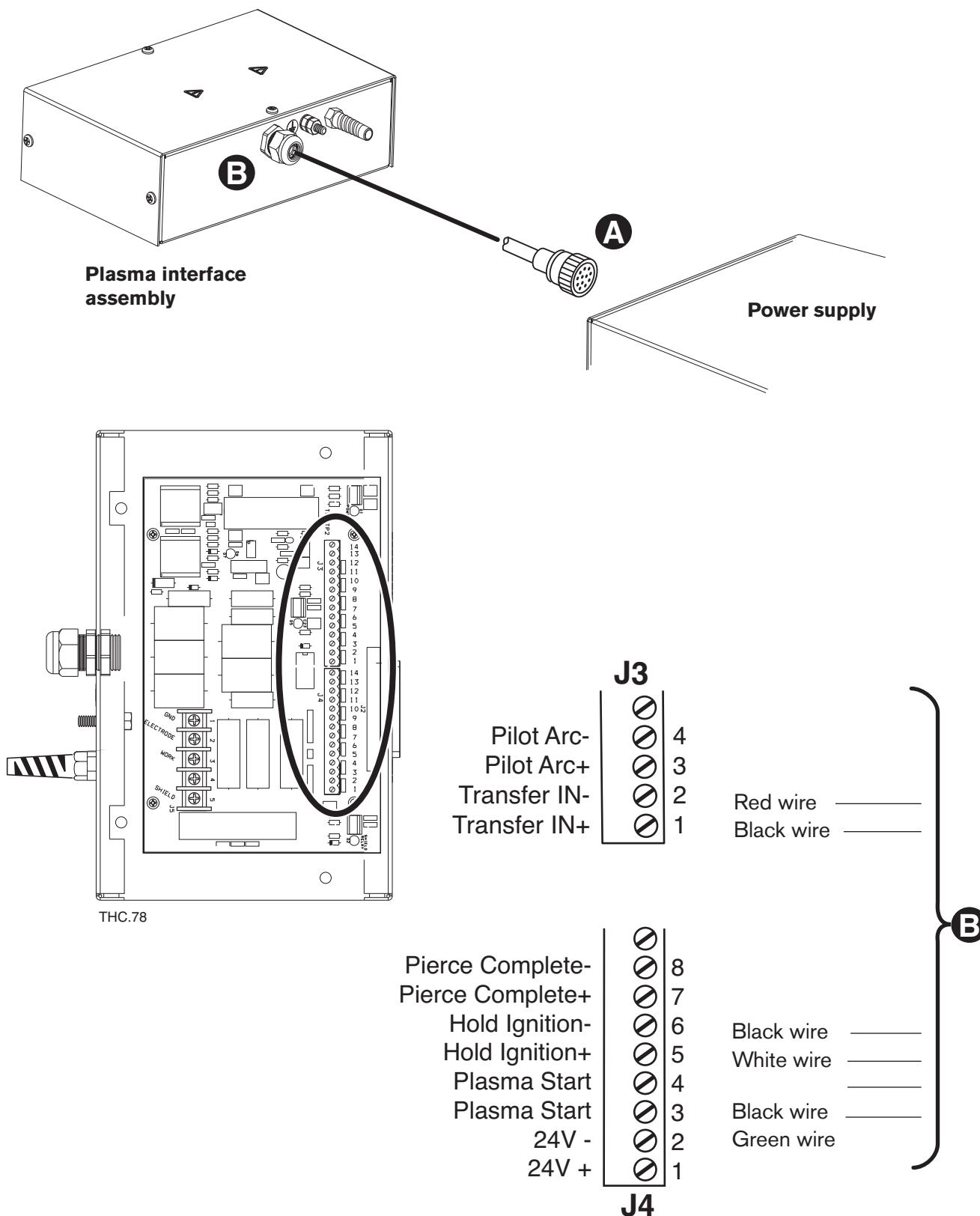
Figure 3f-2 MAX200 power supply interface cable connections
