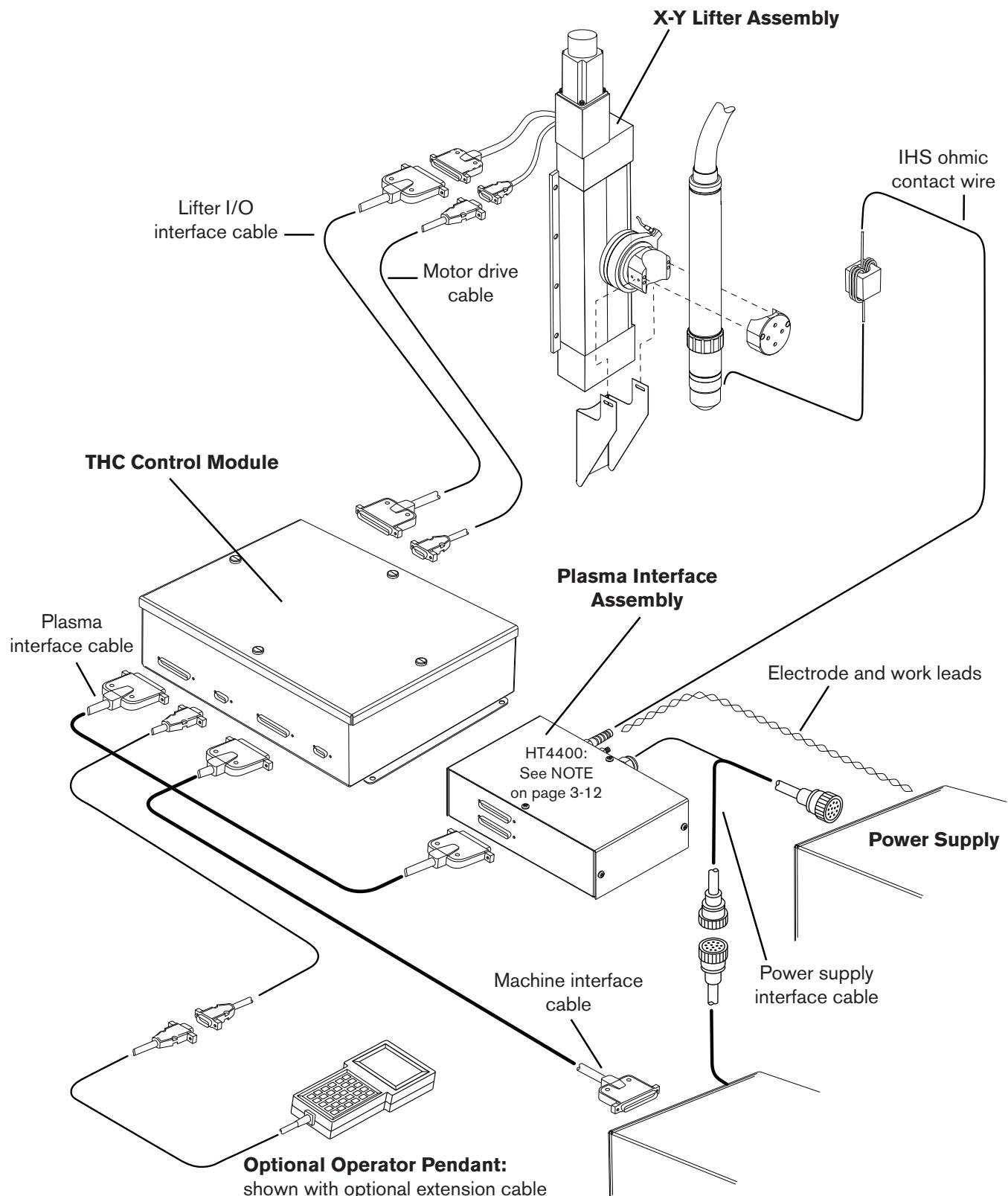
Figure 3-8 X-Y THC system diagram
