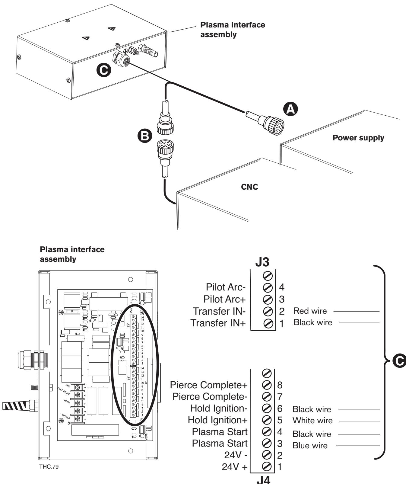
Figure 3b-2 HT2000 power supply interface cable connections
