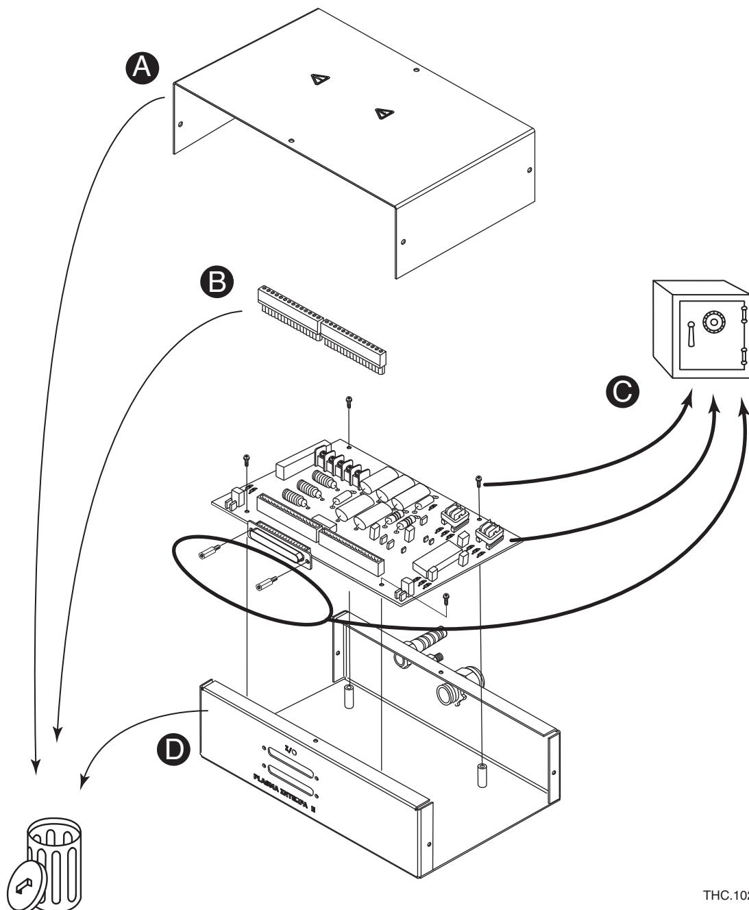
Figure 3h-1 Plasma interface PC board preparation
