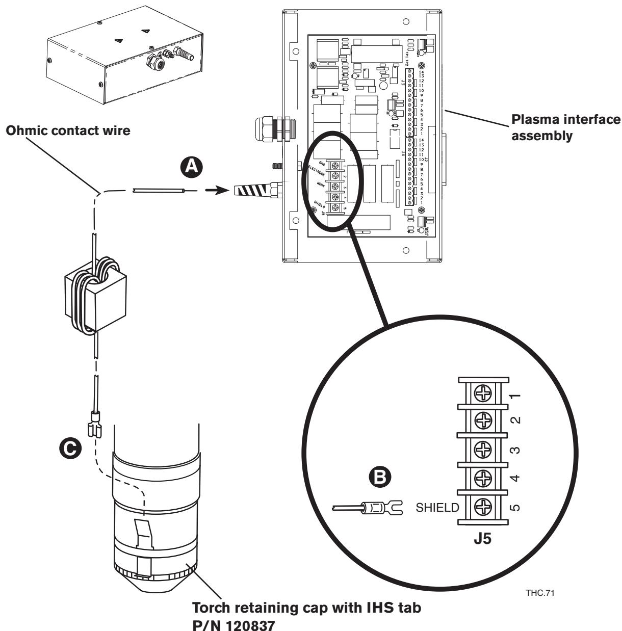
Figure 3b-4 HT2000 ohmic contact wire connection
