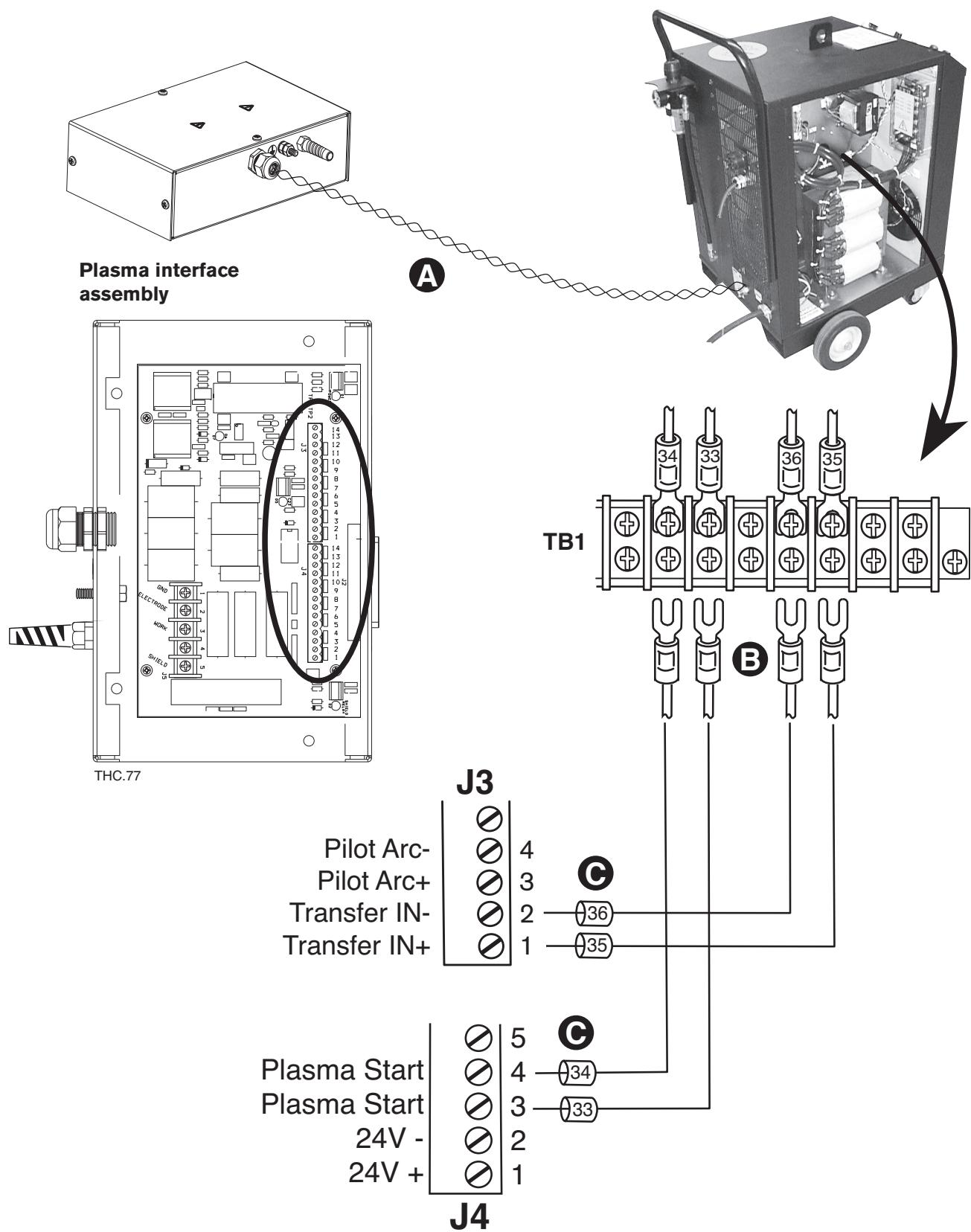
Figure 3e-2 MAX100 power supply interface cable connections
