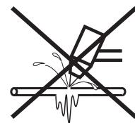
**A PLASMA ARC CAN DAMAGE FROZEN PIPES**
