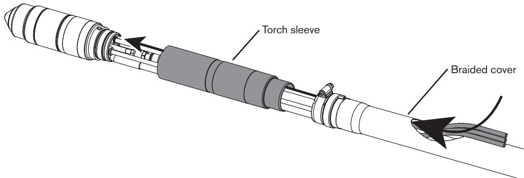
2. Insert the connector into the torch receptacle and turn it by hand until it is tight.
