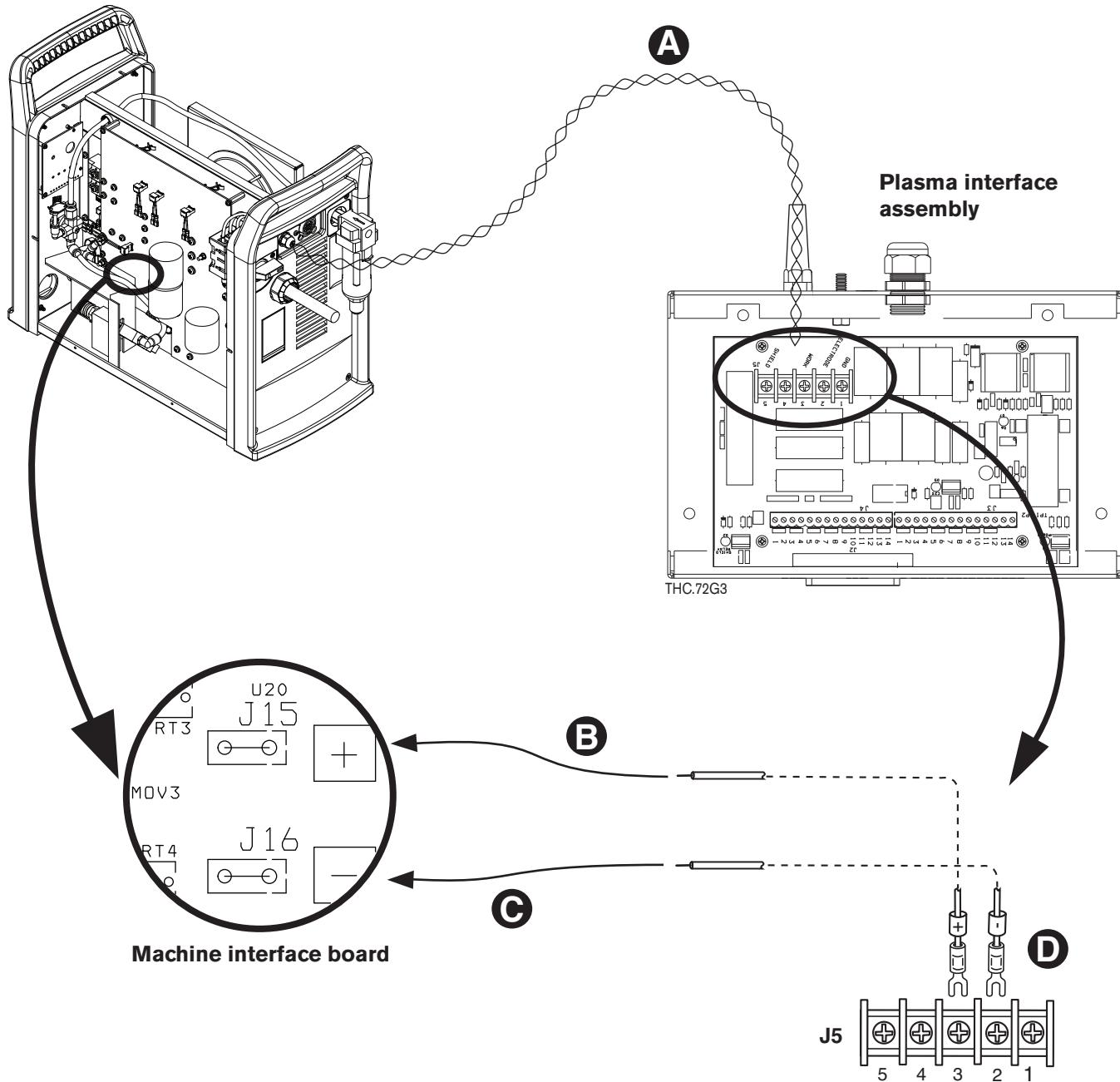
**Figure 3g-2 Powermax1000, Powermax1250 and Powermax 1650 electrode and work lead arc voltage wire connections**
