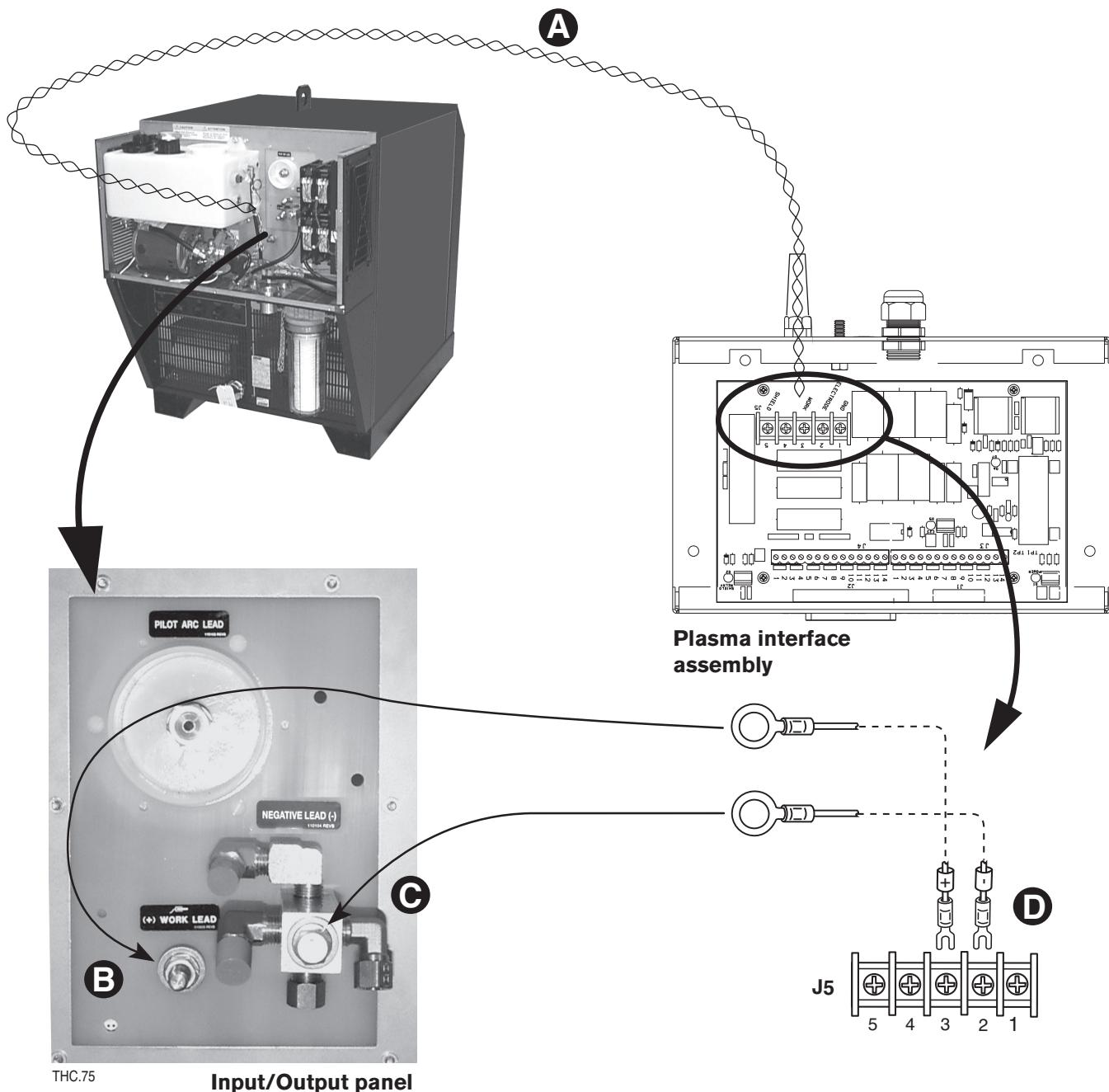
Figure 3c-1 HT2000LHF electrode and work lead arc voltage wires connection
