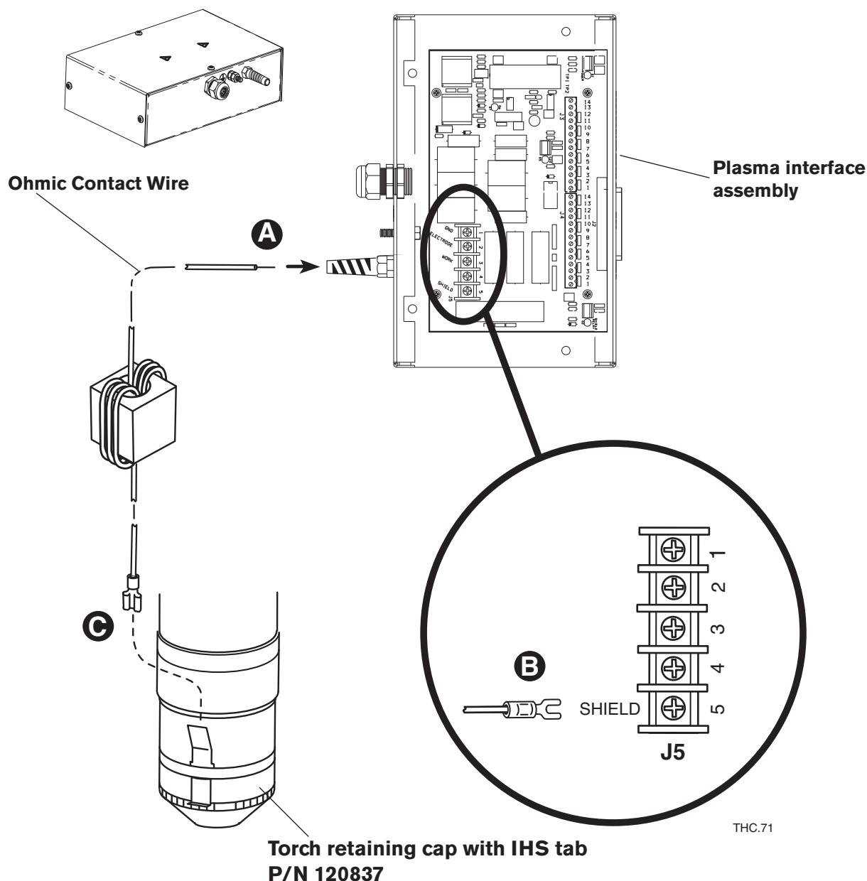
Figure 3f-4 MAX200 ohmic contact wire connection
