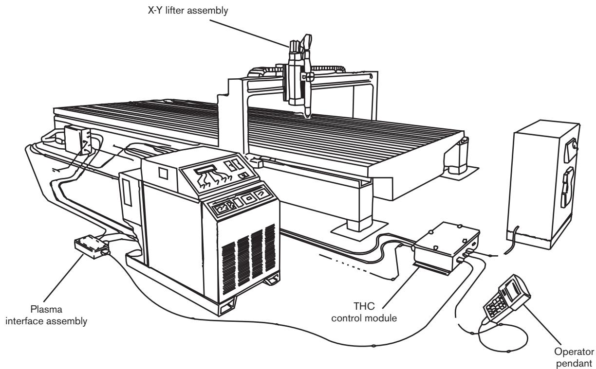
**Figure 2-1 X-Y CommandTHC system
