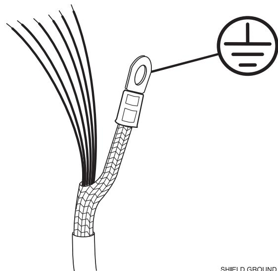
**Figure 3-12 Machine interface cable grounding**
