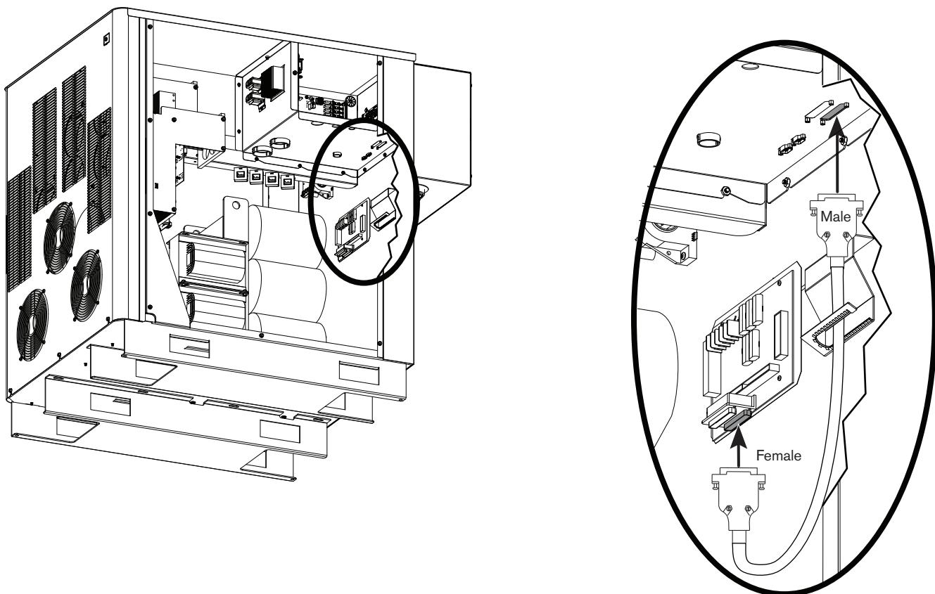
**Figure 3i-10 Plasma interface and control PC board connections**
