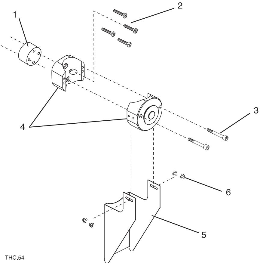
Figure 6-5 X-Y lifter torch mounting block kit
