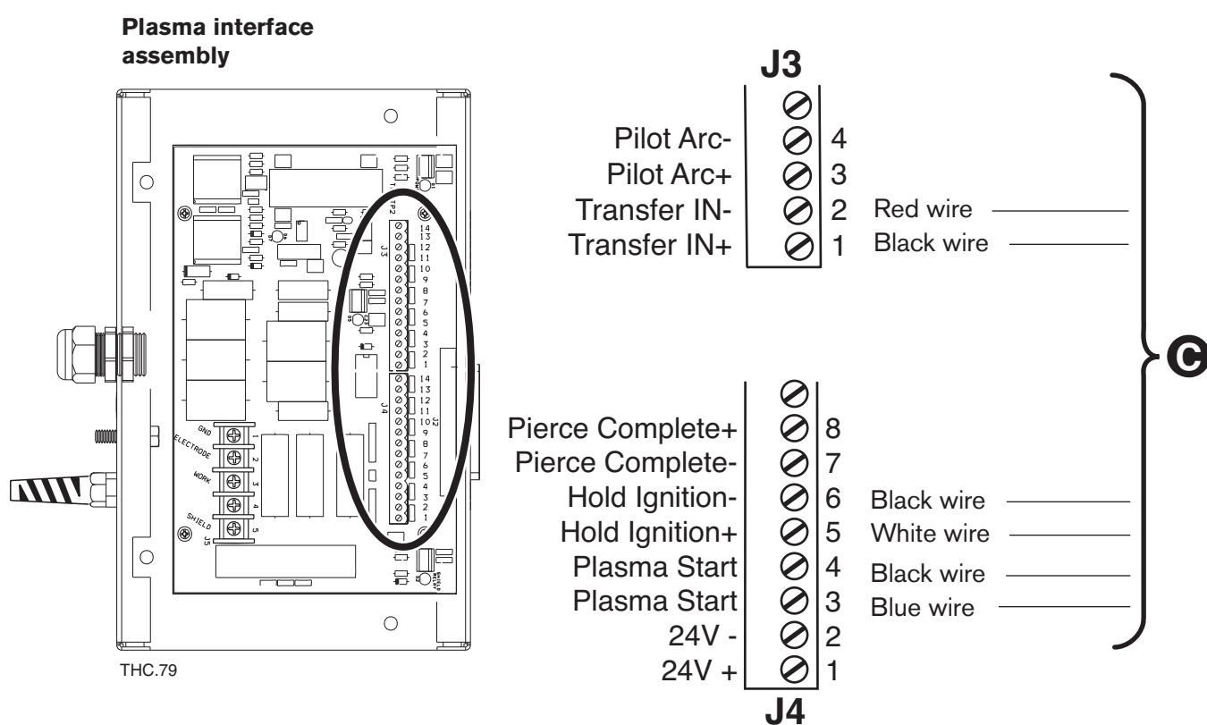
**Figure 3c-2 HT2000LHF power supply interface cable connections**
