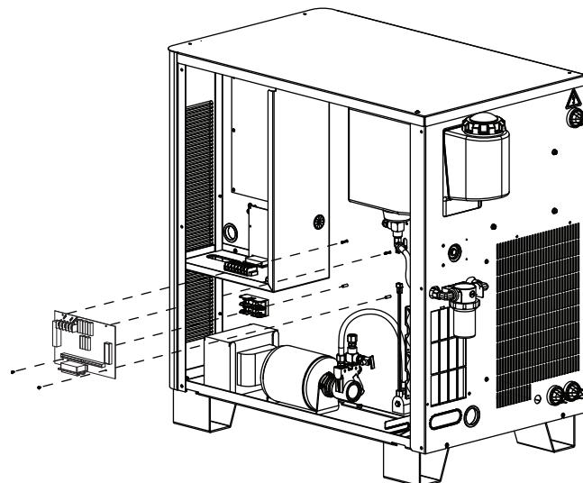
Figure 3i-2 Install the plasma interface PC board
