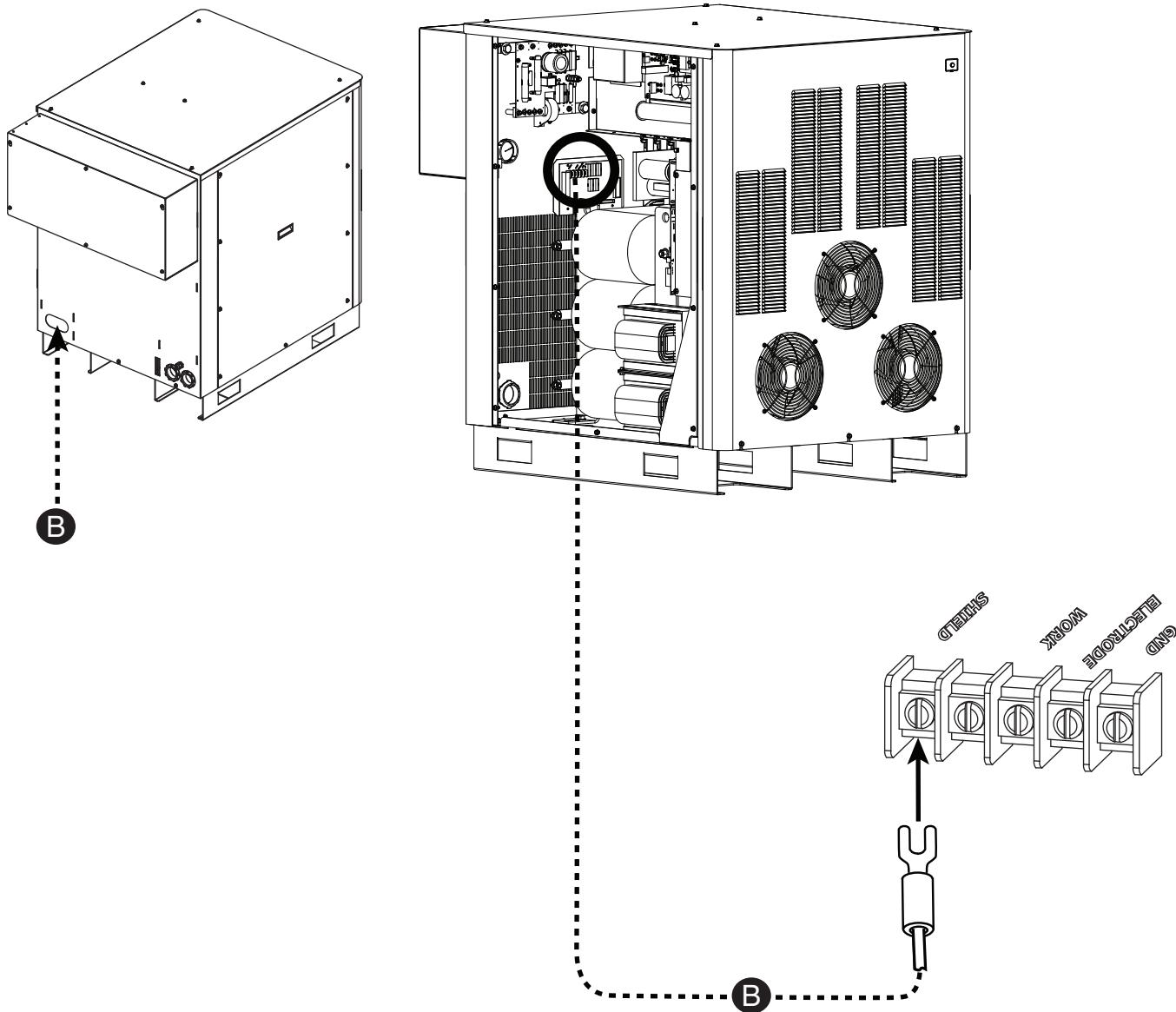
**Figure 3i-14 Ohmic contact wire connection**
