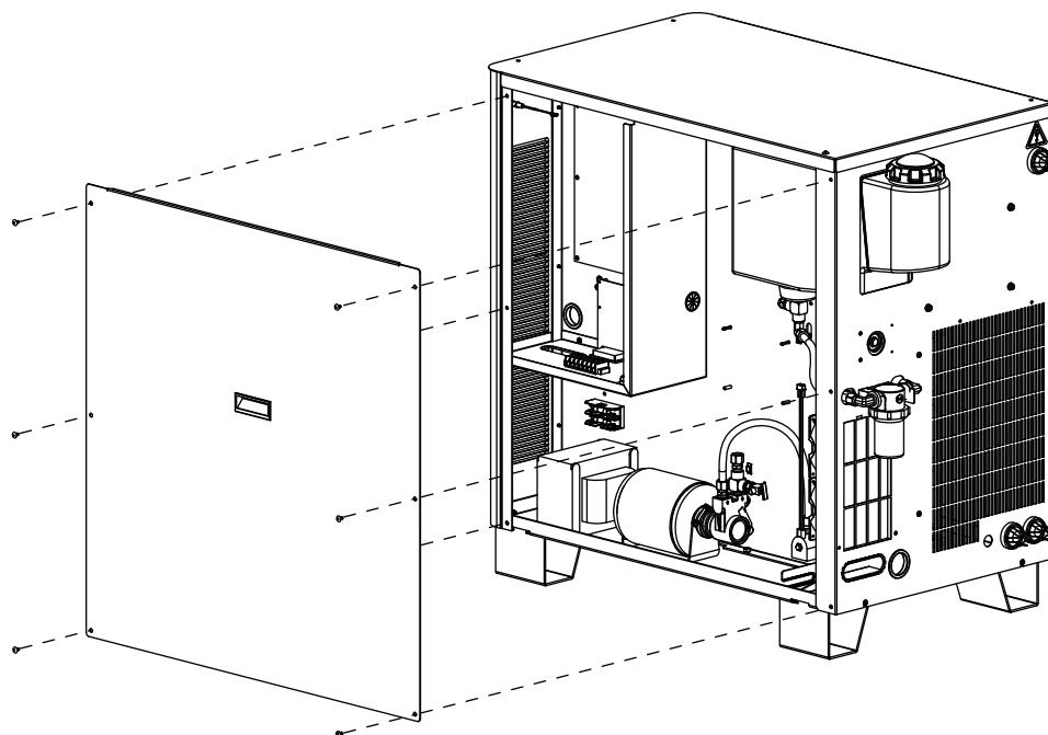
Figure 3i-1 Right side panel removal
