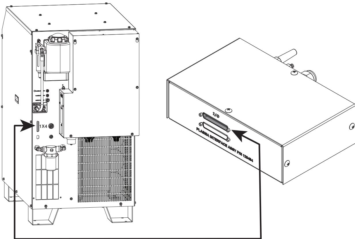
**Connect the plasma interface assembly to the THC control module**
