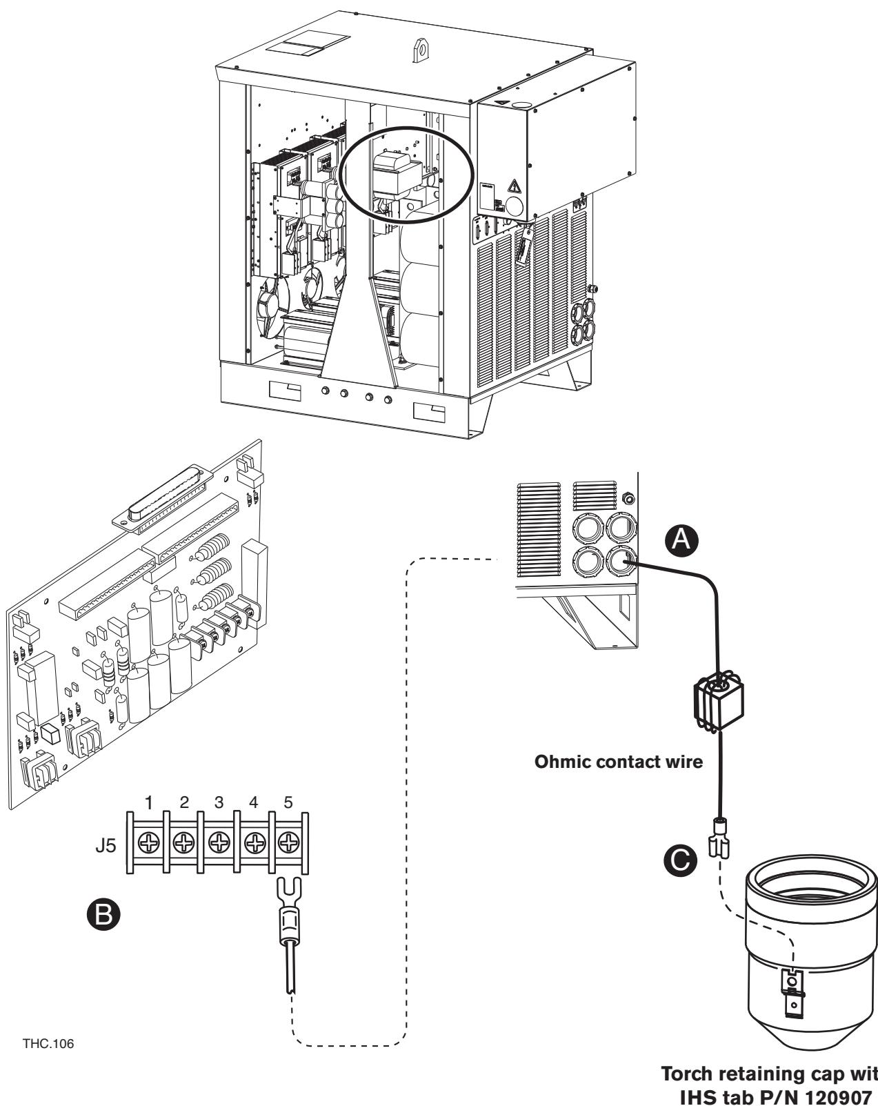
Figure 3h-4 HT4400 ohmic contact wire connection
