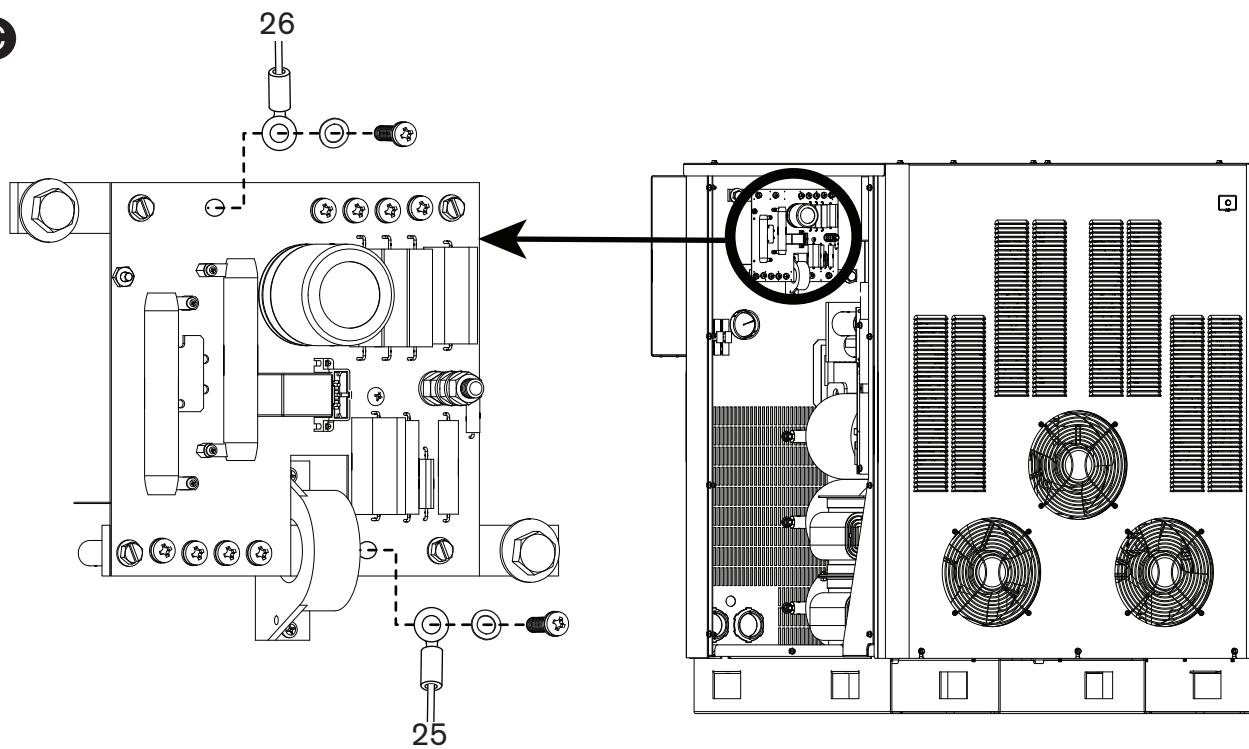
Figure 3i-13 I/O board connections
