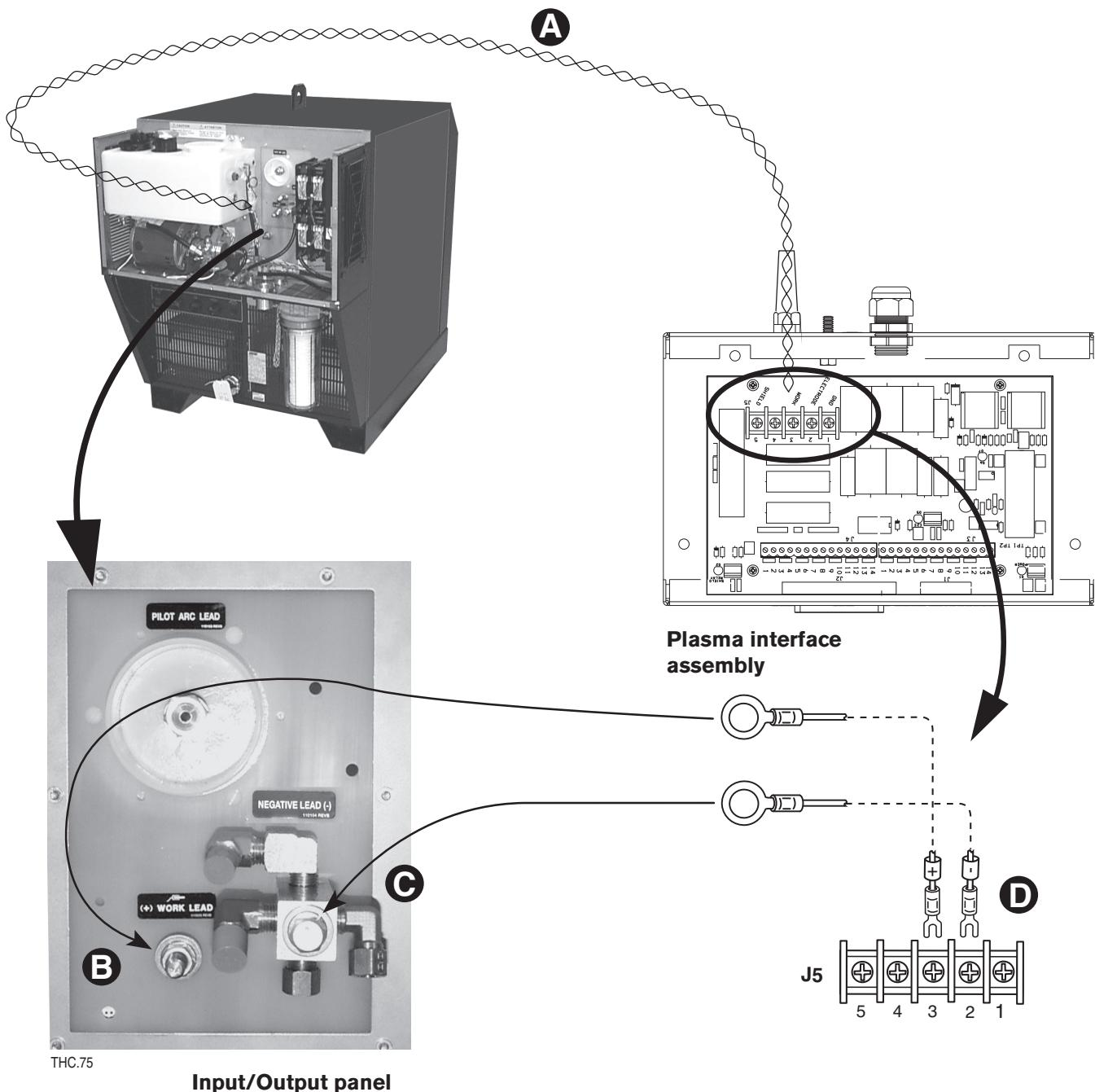
Figure 3b-1 HT2000 electrode and work Lead arc voltage wires connection
