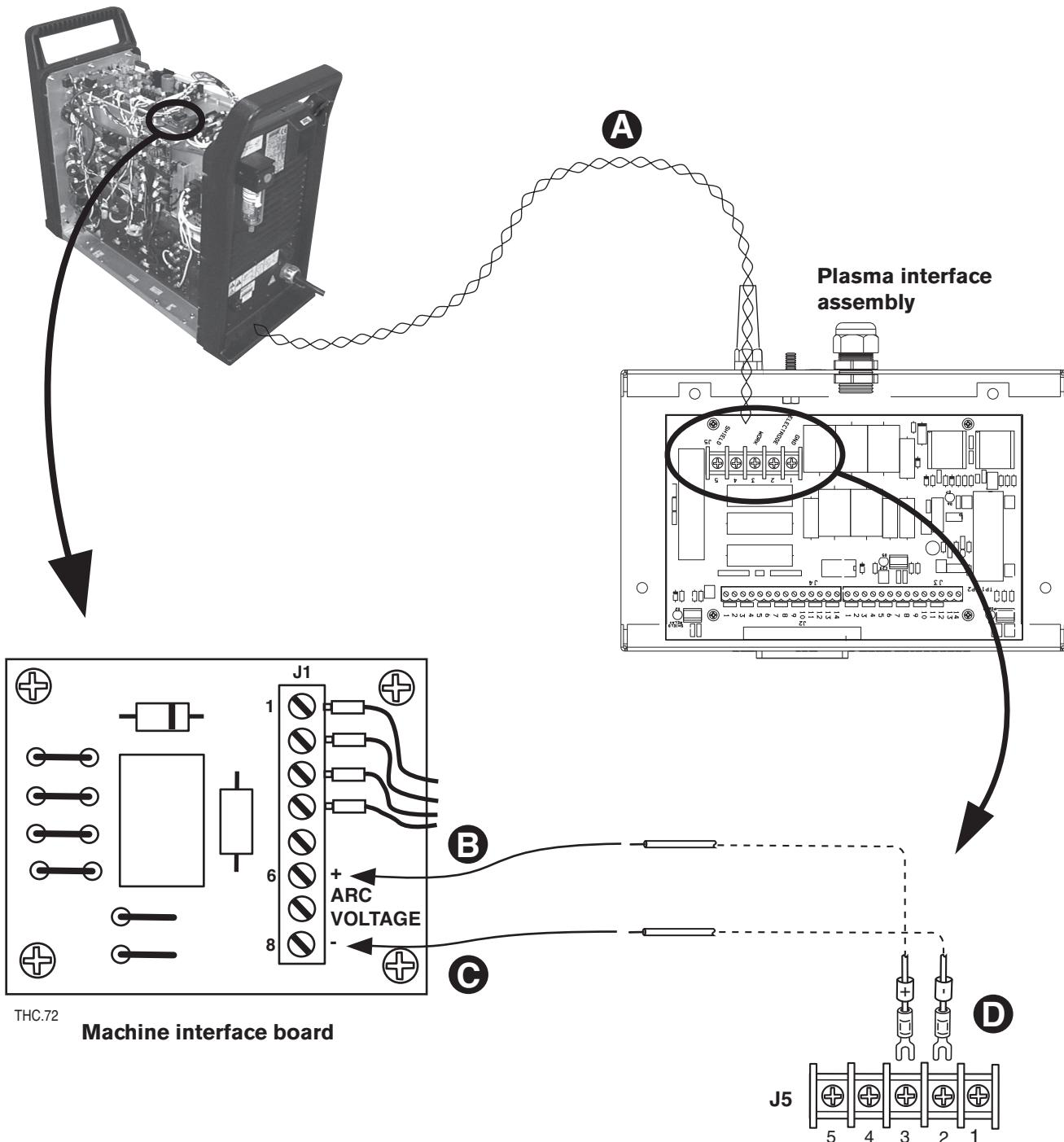
Figure 3g-1 Powermax800, Powermax900 and Powermax 1100 electrode and work lead arc voltage wire connections
