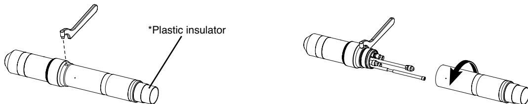
3. Push back the braided cover and slide the sleeve over leads. Align the torch with the hoses in the lead assembly. The hoses must not be twisted. They are taped together to help prevent twisting.
