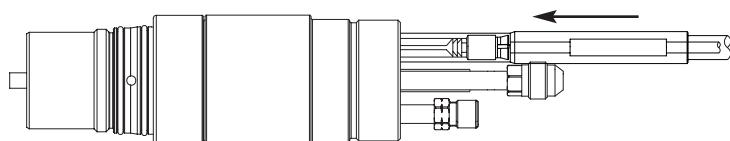
8. Slide the torch sleeve over the connections and screw it onto the torch body.
