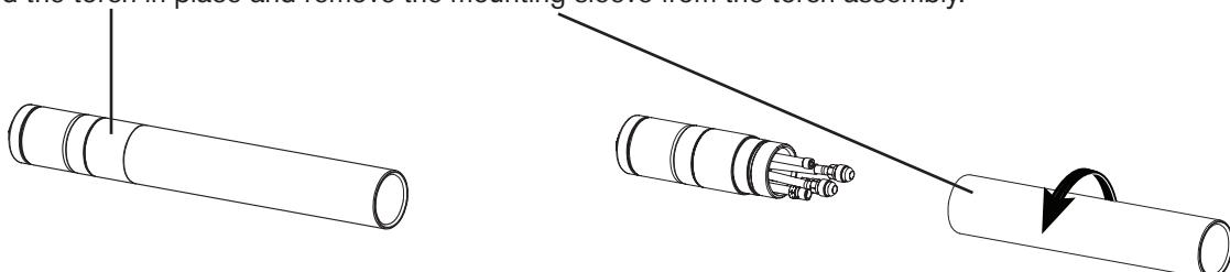
3. Push back the braided cover and slide the sleeve back over the leads. Align the torch connections with the hoses in the lead assembly. The hoses must not twist, and they are taped together to help prevent twisting.
