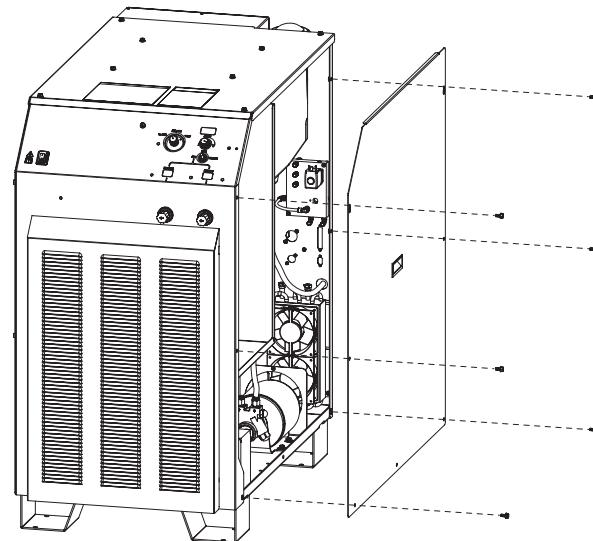
2. Locate the coolant drain valve and use a 20 liter (5 gallon) container to catch the coolant. Coolant will flow as soon as the drain is opened. Close the drain valve when the coolant stops flowing. Always dispose of coolant according to local and national codes.
