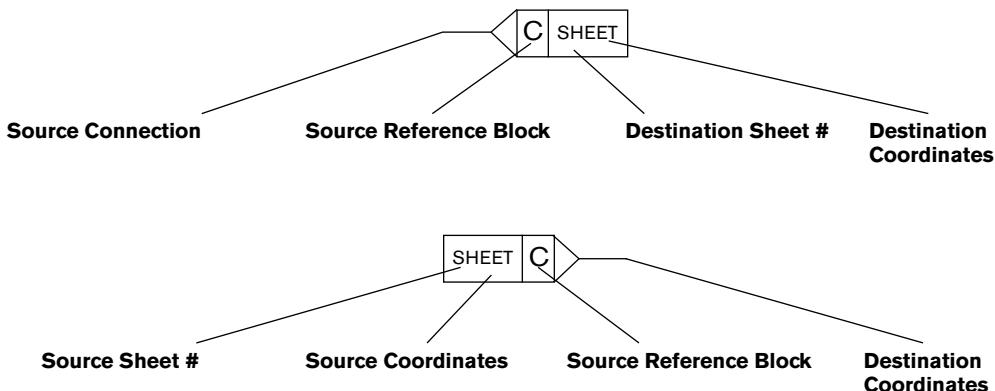
**Destination** and **Source Coordinates** refer to letters A-D on the Y-axis of each sheet and numbers 1-4 on the X-axis of each sheet. Lining up the coordinates will bring you to the source or destination blocks (similar to a road map).
