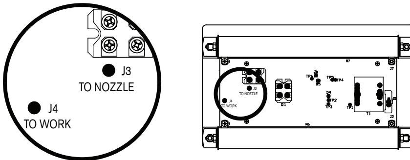
4. Measure the ohm value between the nozzle and the plate. The reading should be < 3 ohms. A measurement > 3 ohms indicates a faulty connection between the torch and ignition console, or between the ignition console and the power supply.
