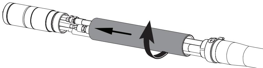
9. Slide the braided cover up to the torch sleeve. Push the brass collar into the torch sleeve. It is a snug fit. Make sure the plasma and shield hoses are routed through the hole in the braided cover.
