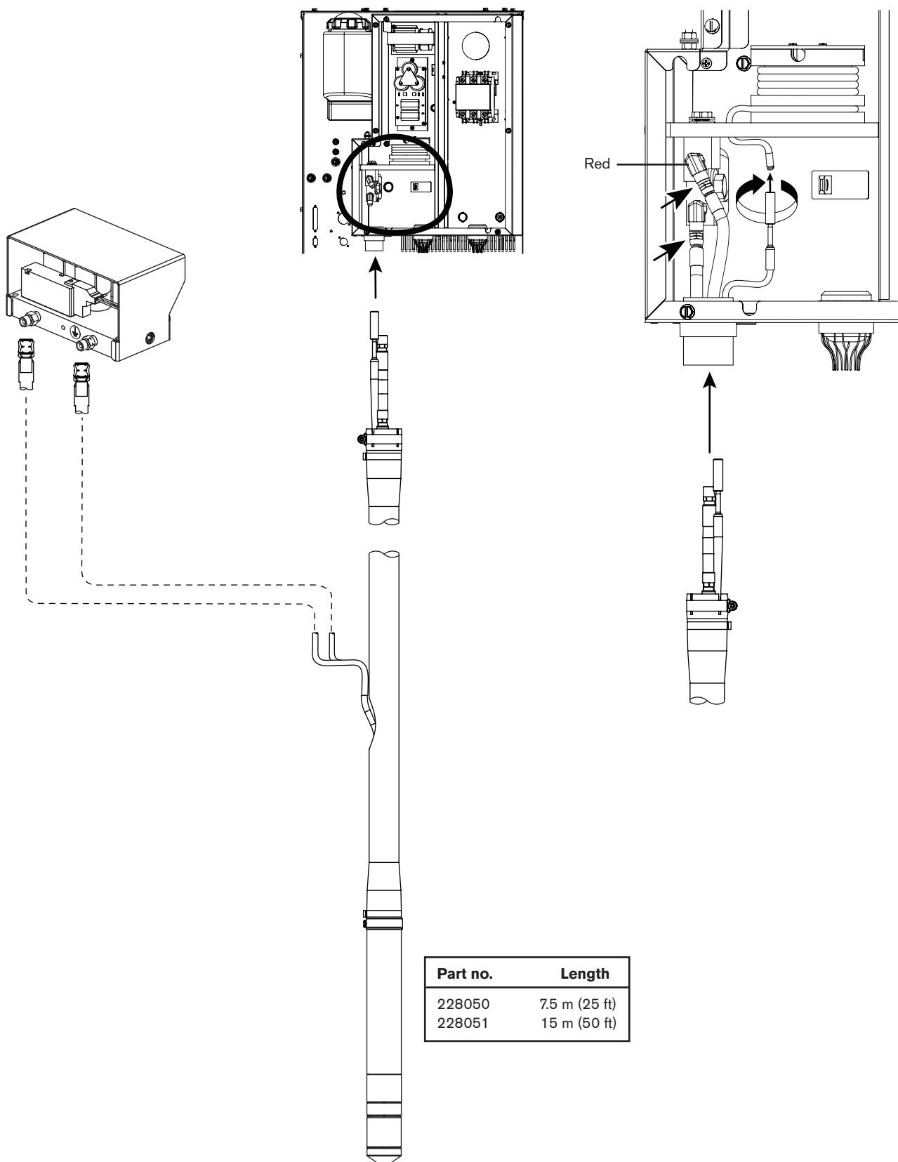
**Connect the torch to the torch lead assembly**
