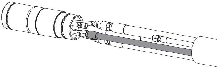
6. Connect the plasma gas hose. This connection has left-hand threads.
