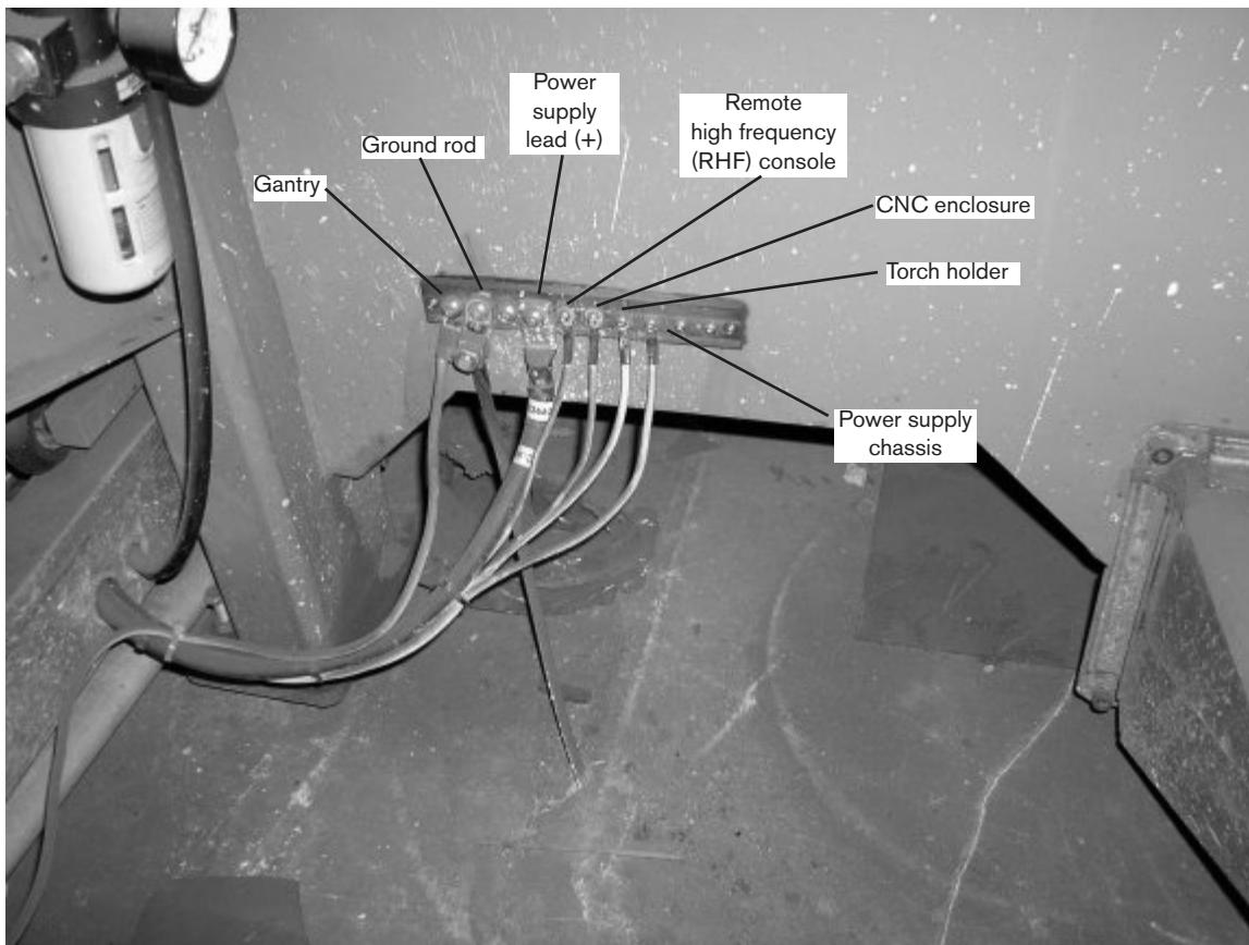
Example of a good cutting table ground bus. The picture above shows the connection from the gantry ground bus, the connection from the ground rod, the power supply positive lead, the RHF console\*, the CNC enclosure, the torch holder, and the power supply chassis.
