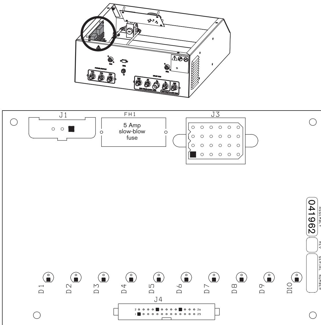
**Gas console AC valve driver board LED list**
