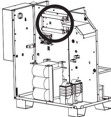
3. Install a temporary jumper wire between J4 (work) and J3 (nozzle) on the start circuit PCB1.
