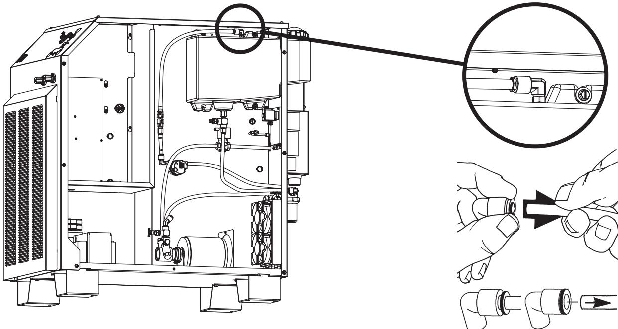
3. Turn ON the power and have another person push and hold the current knob, to override the flow time-out error. Allow the coolant to flow for 45 seconds, and turn OFF the power.
