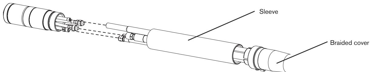
4. Connect the coolant hoses to the torch. Red connects to red. Use 2 wrenches to tighten gas and coolant fittings.
