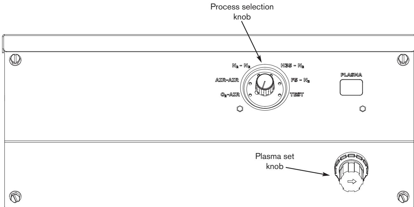
Note: The plasma set knob on the fuel-gas console is used when an H35 or F5 process is selected. The plasma set knob on the power supply is used (as described on the previous page) when an O<sub>2</sub>, Air, or N<sub>2</sub> process has been selected.
