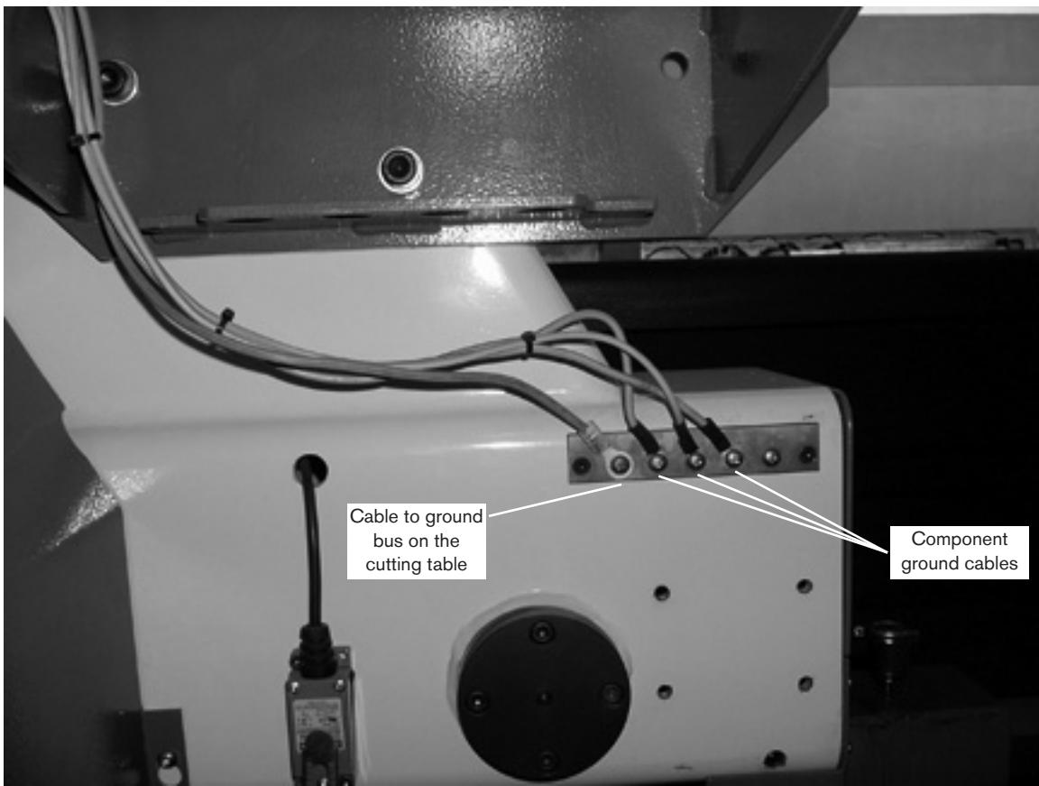
Example of a good gantry ground bus. It is bolted to the gantry, close to the motor. All of the individual ground cables from the components mounted on the gantry go to the bus except those from the RHF console\* and the torch holder. A single heavy cable then goes from the gantry ground bus to the ground bus bolted to the table.
