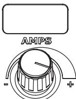
If Channel 1 passes the test, the system will repeat the test for channel 2 and current sensor 2. Error code 075 will show in the AMPS display if the current is < 10 amps. Error code 107 will show in the AMPS display if the current is > 35 amps.
