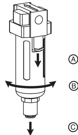
Use a screwdriver to remove the filter element from the filter housing. Then install the new filter element.
