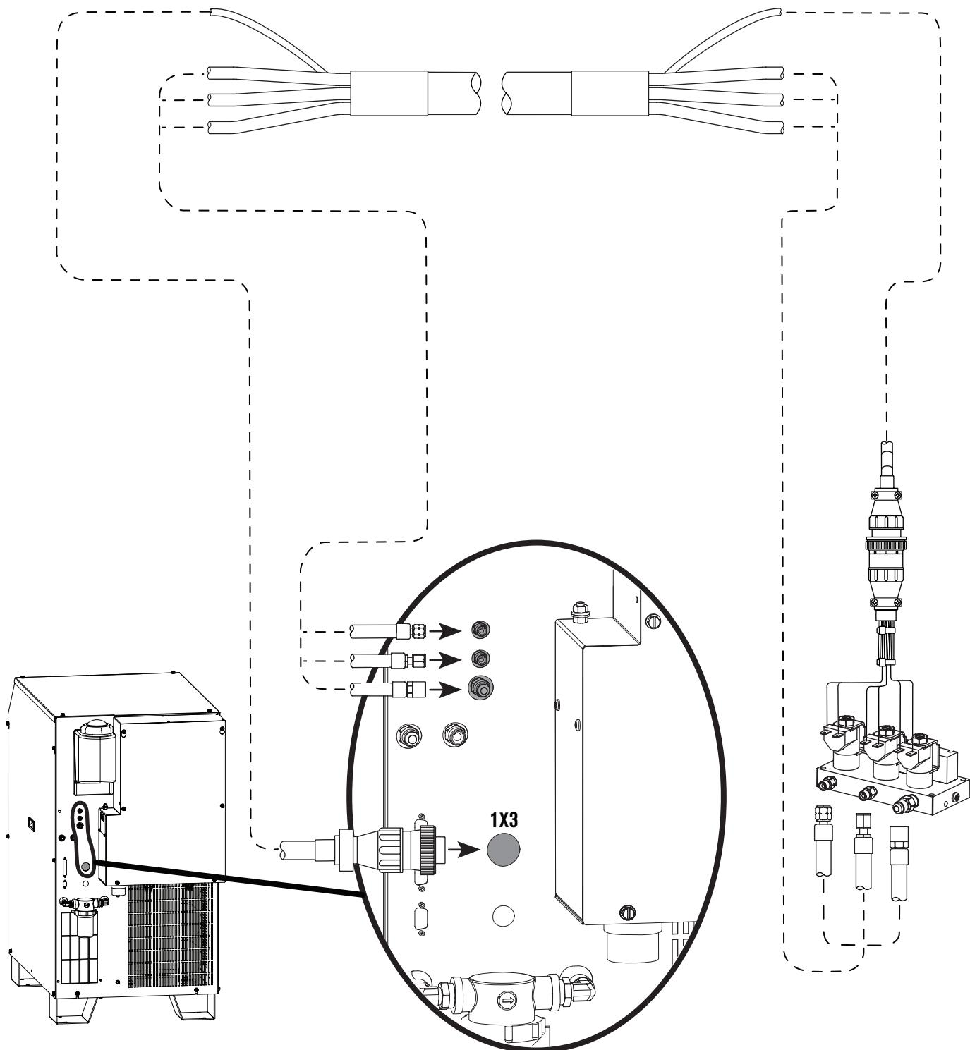
**1a Fuel gas console to off-valve connections**
