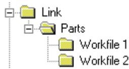
Any part programs to be viewed and downloaded at the control would be placed here. Only the sub folders Workfile 1 and Workfile 2 and the program files located within them will be viewed at the control.
