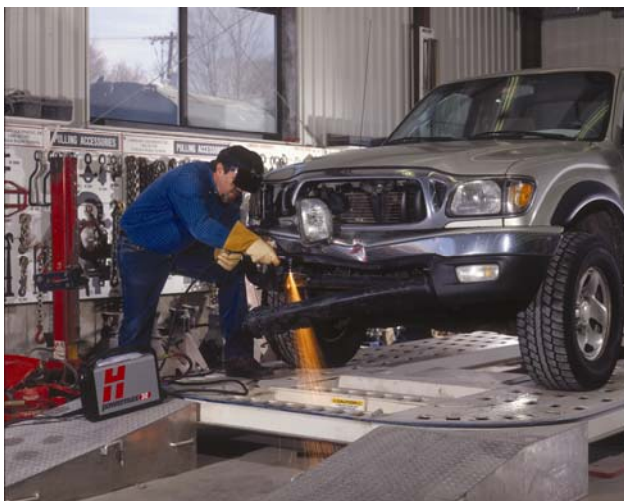
Manual plasma systems are most commonly used in the automobile repair, construction, and metal art industries.
