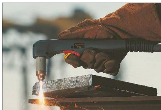
Plasma does a good job of cutting thick plate as shown in this photo
