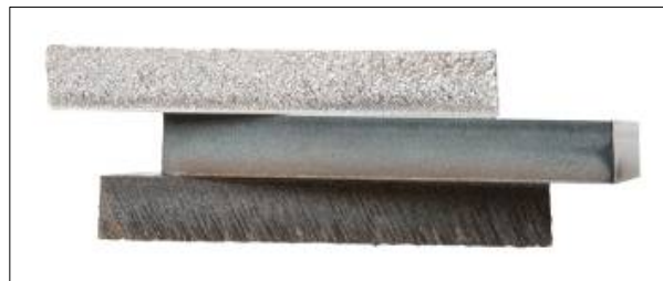
Plasma cuts mild steel, stainless steel, aluminum and any other electrically conductive metal.
