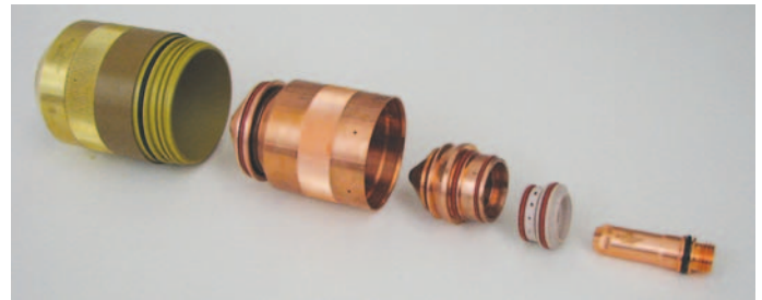
▲ FIGURE 1 All torch components should be regularly inspected, including (from left to right) the outer retaining cap, shield, inner retaining cap, nozzle, swirl ring, and electrode.
