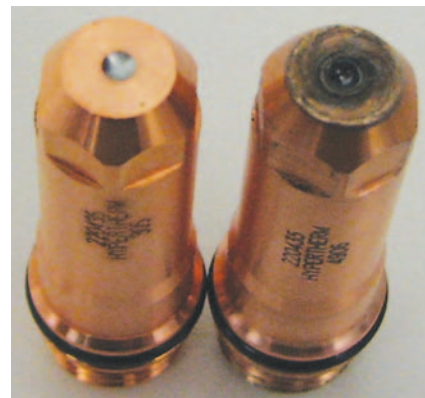
▲ FIGURE 3 The electrode on the right has a pit 0.023 in. deeper than the new electrode on the left. The pit was caused by hafnium evaporation during starting and steady-state cutting.
