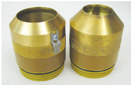
▲ FIGURE 9 The outer retaining cap holds the shield in place over the inner retaining cap and directs secondary gas flow to the shield.
