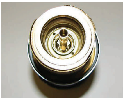
▲ FIGURE 10 Inspect and clean the torch body at least once per shift.
