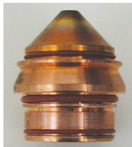
▲ FIGURE 5 The nozzle's primary function is to constrict the plasma gas to increase energy density and velocity.
