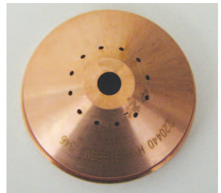
▲ FIGURE 7 The shield protects the nozzle from double-arcing from the workpiece.
