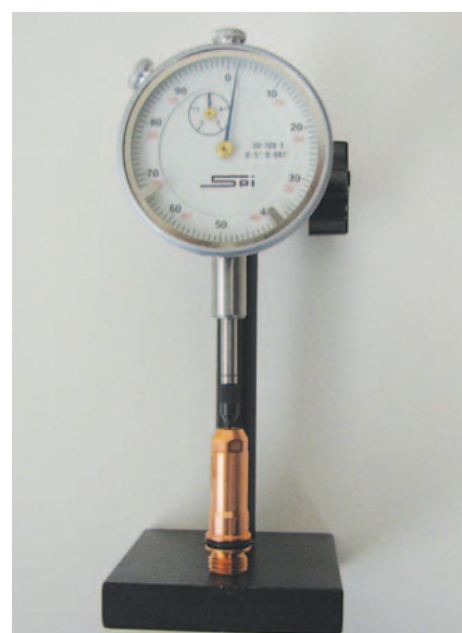
▲ FIGURE 4 Use a dial indicator to measure pit depth of partially used electrodes.
