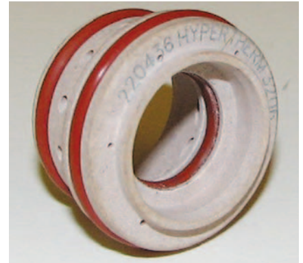
▲ FIGURE 6 The swirl ring swirls the plasma gas flow around the electrode and nozzle, and it creates a centrifugal effect that slings heavier, un-ionized gas molecules to the edges of the nozzle orifice.
