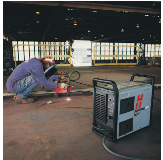
A shipyard employee in North Kingstown, R.I., uses plasma cutting on a track system.
