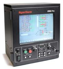
Compatible with nearly any mechanized system, the EDGE Pro is easy to install, easy to use, and more reliable than any other computer numeric control. It does not require any sort of intermediary device to run and supports both oxyfuel and conventional plasma cutting systems.
