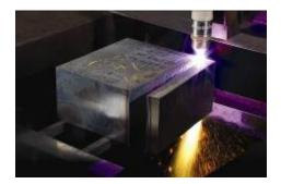
The new HyPerformance HPR800XD® system's thick piercing capability is attributed to PowerPierce<sup>™</sup>. This patent pending technology eliminates the need for pre-drilling and minimizes damage to the torch by using a liquid cooled shield to repel molten metal during piercing and cutting. In testing, Hypertherm found there was no damage to its consumables or lessening of cut quality, even after piercing 3" (75mm) thick stainless steel 400 times.
