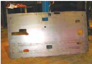
Platform cutout for an excavator cab. One of Wrayco's many jobs now fabricated using HyPerformance Plasma.
