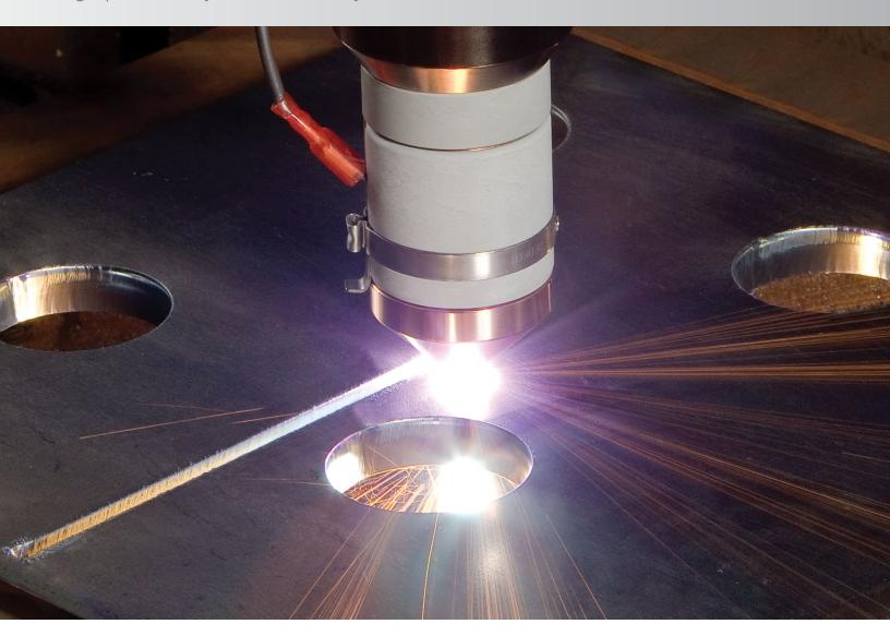
The New HyPro2000 for the HT2000 provides increased productivity through 50% faster speeds, 75% longer life and a quick-disconnect torch.
