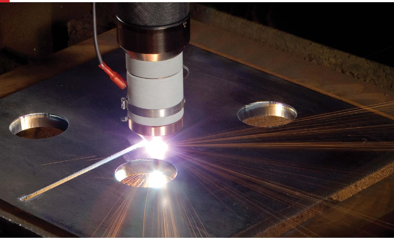
The New HyPro2000 for the HT2000 provides increased productivity through 50% faster speeds, 75% longer life and a quick-disconnect torch.
