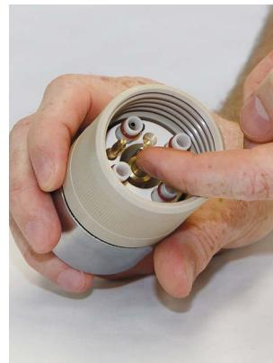
The proper amount of grease will leave the o-ring "shiny", but leave no excess or built up grease. Excess grease will attract contaminants and could cause restrictions in critical passages. Grease may be applied either by finger or using a cotton swab. Always replace o-rings if they have cracks or tears. If you are replacing a water tube remember to lubricate the small o-ring on the base of the water tube.
