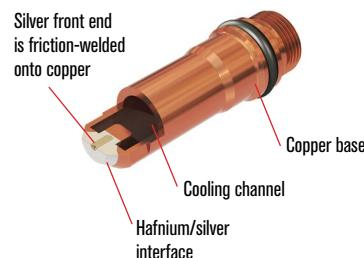
**TrueFlow™** allows for centered electrode alignment with the water tube to ensure optimal cooling, which increases life and produces a higher and consistent cut quality.
