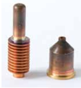
Partially used electrode and nozzle
