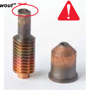
Overused electrode and nozzle
