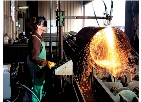
Pipe cutting and beveling
