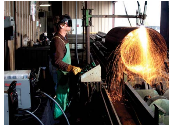
Pipe cutting and beveling
