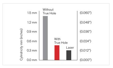
Example based on 10 mm holes, 9.5 mm mild steel plate, 130 A process (0.394" holes, 3/8" mild steel plate)
