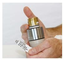
Apply a thin film of silicone lubricant on each external o-ring.
