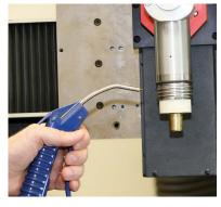
Use compressed air to blow off the coupler threads.
