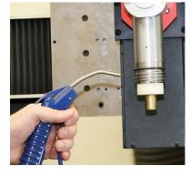
Use compressed air to blow off the coupler threads.
