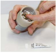
Inspect each of the 5 o-rings at the rear of the torch for nicks and cuts. Replace any damaged o-rings. If they are not damaged, apply a thin film of silicone lubricant on each o-ring. The o-rings should look shiny, but there should not be any excess or built-up grease.
