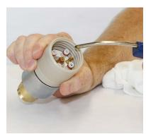
Use compressed air to blow off all internal surfaces.
