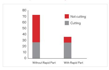
In this example, non-cutting time (red) is reduced by 80%, lowering the overall production time by 50%.
