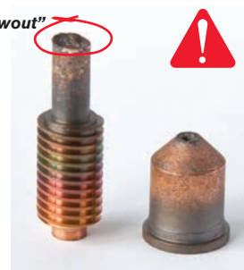
Overused electrode and nozzle
