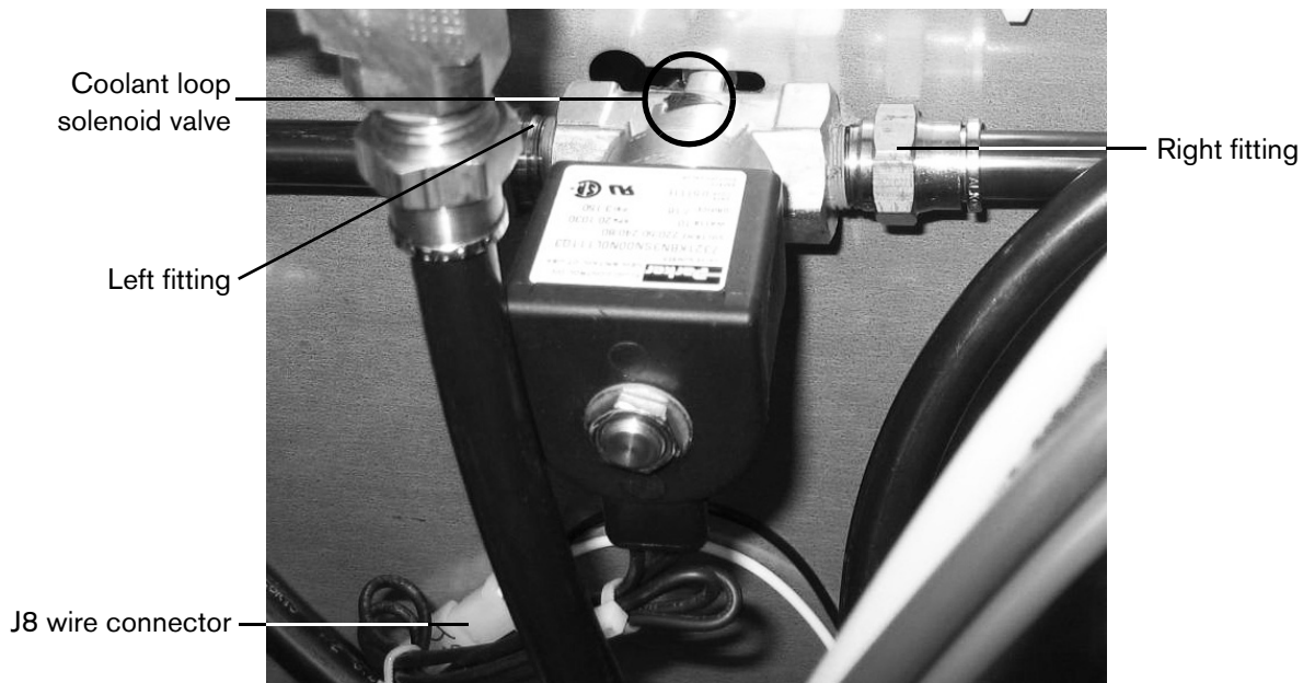
Figure 6: Coolant loop solenoid valve correctly positioned within the HSD130 power supply
