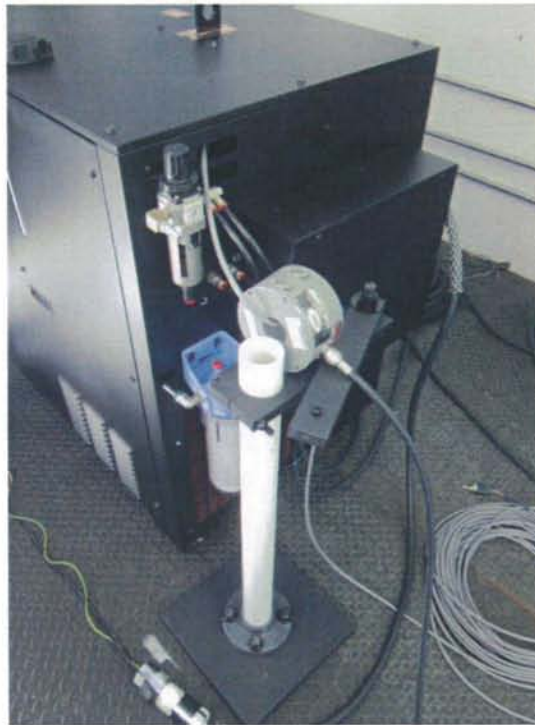
I/O Port Test Configuration, Bulk Current Injection
