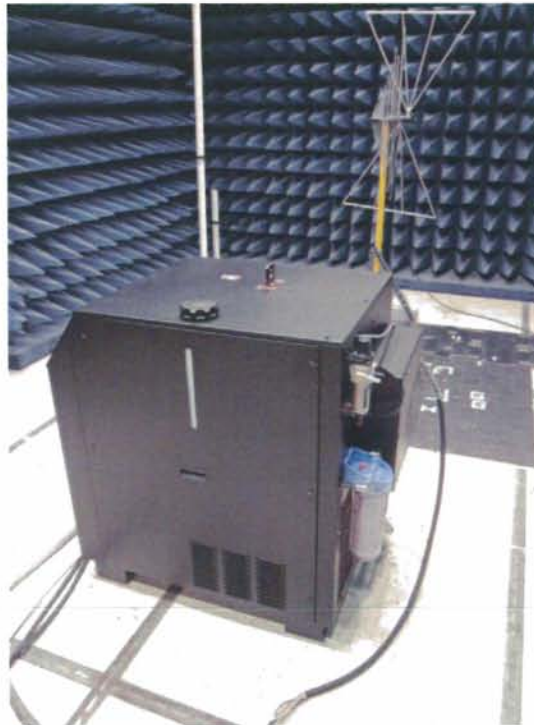
Vertical Antenna Polarization, 80 MHz to 1 GHz
