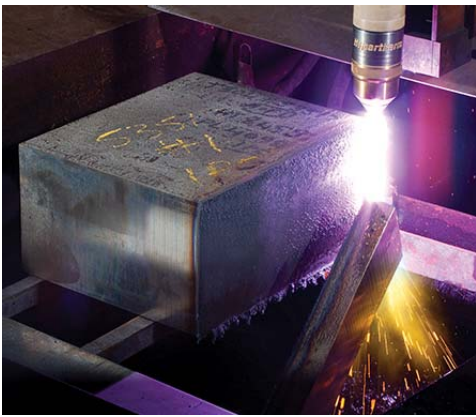
Figure 3 – Example of dogleg lead-out programmed cut path
