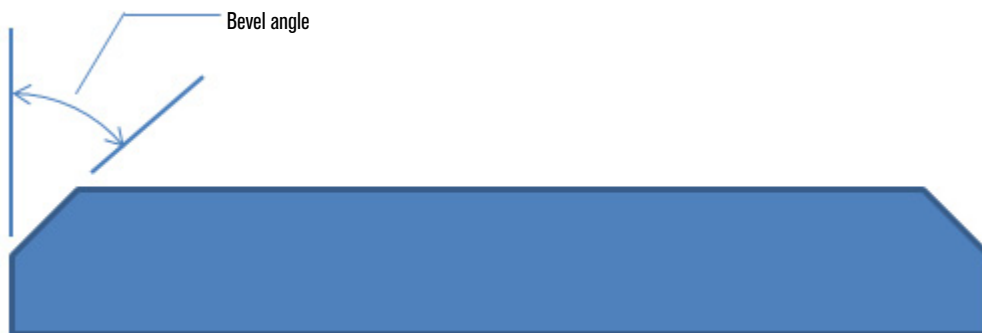
Figure 28 – Y Top cut bevel angle
