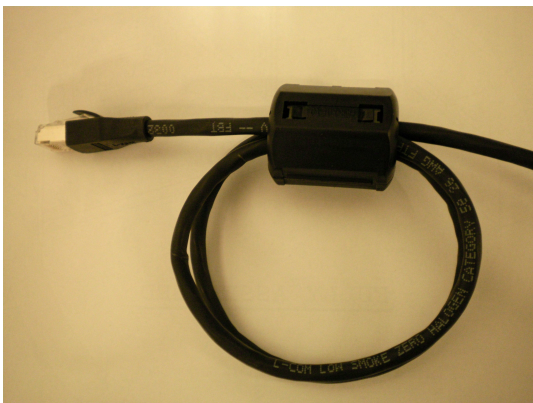
Figure 53 Ferrite filter installed on a Hypernet or LAN cable
