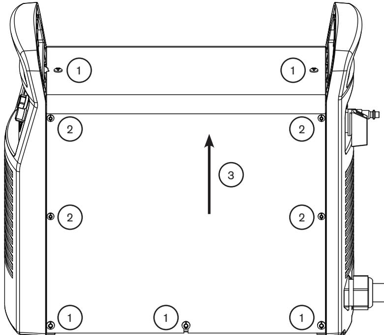
5. Remove the Mylar barrier from the power-board side of the power supply. The Mylar barrier is flexible and can be bent slightly for removal.
