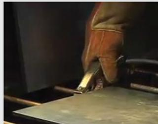
**Do not attach clamp to a portion of the workpiece that will fall away.**
