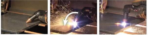
Gouging | Gougeage | Ranurado
