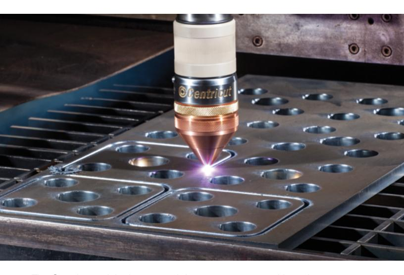
The Centricut quick-change torch incorporates proven Hypertherm technology to deliver excellent performance, improved productivity and high reliability for your ESAB cutting system.
