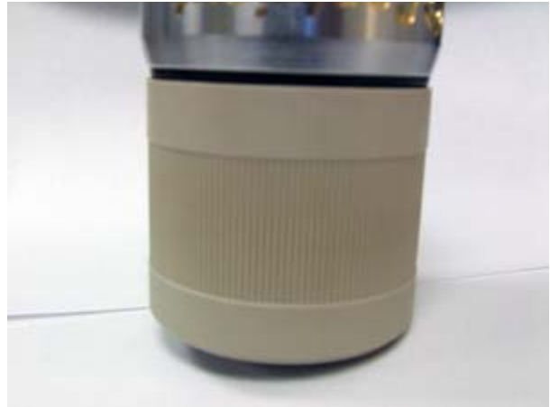
Improperly installed mounting nut
