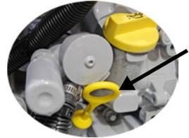
**c. Check the oil level in the air compressor.**
