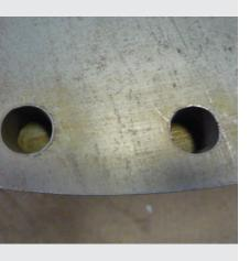
Each 3/4" thick part has 46 bolt holes that required an hour to drill. With plasma, it takes 12 minutes
