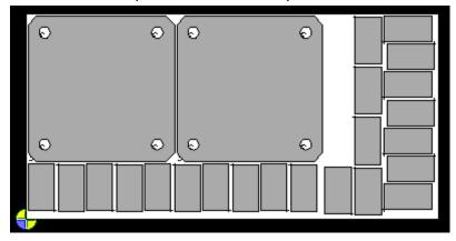
Nesting can be done manually, where parts are added to the plate one at a time. A part or group of parts can also be arrayed onto a nest. Nesting can also be done automatically.
