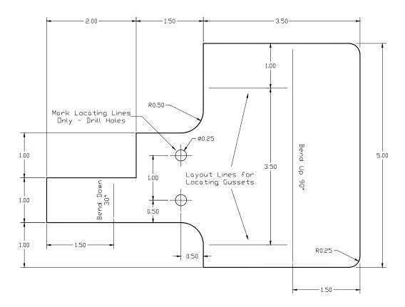
**TASK - Processing:** For this task ensure that the Hypertherm plasma machine set-up has been selected. Import the drawing into ProNest and assign the following parameters: Quantity 5, Material MS, Thickness 0.500 in., Class 130 Amp  $0_2$ /Air (True Hole).
