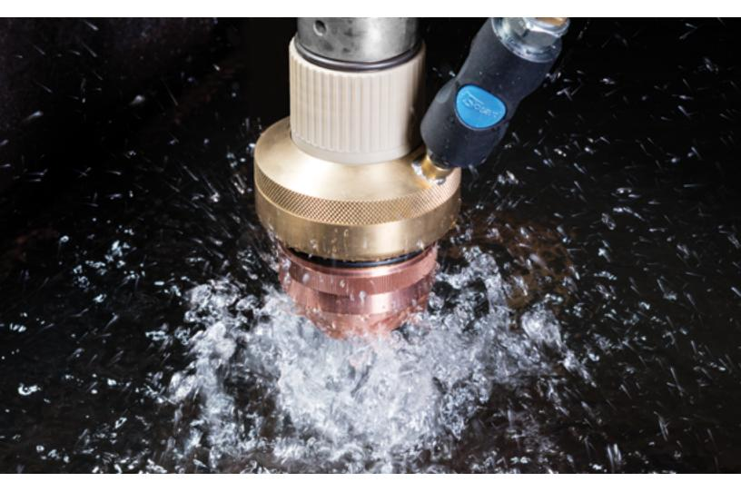
The Centricut air curtain delivers ease of use and reliability to your underwater cutting process.
