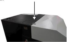
2. Disconnect the high-pressure tubing from the right end of the attenuator. The tubing and connections are shown in red.
