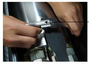
3. Put the guard straps over the tabs on the top of the attenuator guard.
