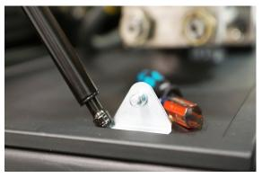
5. Remove the mounting bolts at both ends of the bridge.
