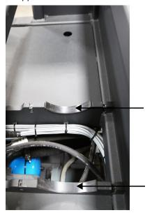
4. Use the attenuator locating tool from the 16323 Attenuator guard installation tool kit to make sure that the attenuator is centered on the supports. Line up the notched end of the tool with the flat face of the attenuator body. The attenuator is centered when the support end of the tool is flat against the attenuator support.
