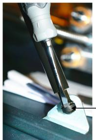
b. Hit the shock with an open hand to release it from the ball.
