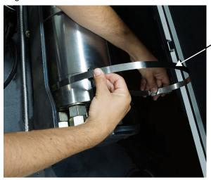
2. Put the ends of the guard straps into the bolt drives.
