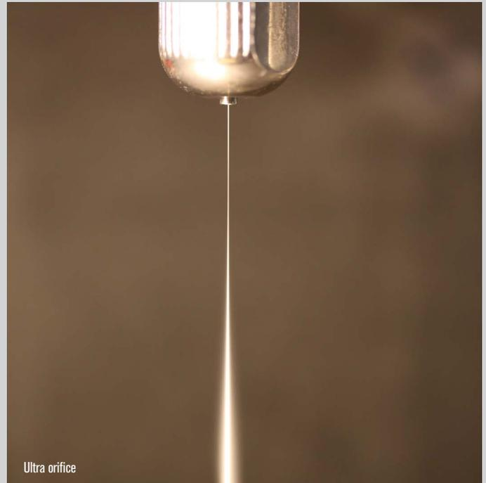
You can see the difference. In side-by-side comparison of 50,000 psi (0.010" orifice) waterjet streams, the new Ultra orifice shows significantly better definition, which translates to improved quality and faster cutting speeds.
