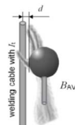
Figure 15 – Field measurement at limb positions, hand and thigh
