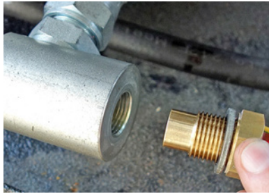
Figure 90 – Temperature switch and washer removed from fitting
