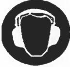
The plasma cutting process can generate high levels of noise. Depending on the arc current, material being cut, acoustics and size of the cutting room, distance from the torch and other factors, acceptable noise levels as defined by local and/or national codes may be exceeded by your plasma system.
