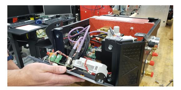
**5.** Disconnect the SV100 connector ③ from the mixer module.
