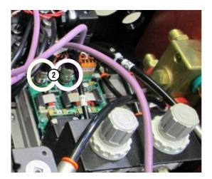
**4.** Remove the manifold-side panel to get access to the mixer module (229703). This manifold-side panel has the 24 V power supply (229640) and control PCB (141375) attached. Refer to Gas connect console panels on page 102.
