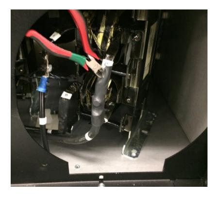
9. Remove the 3 inductor wires from the cable holder.
