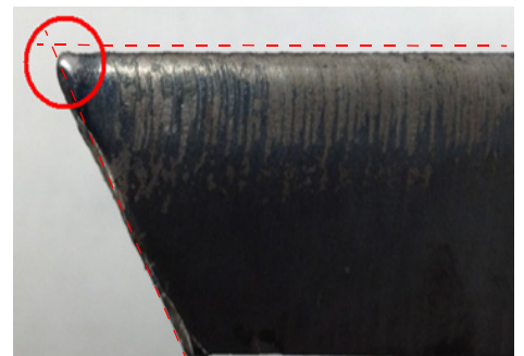
Figure 8 – Part size reduction on an A cut because of top corner rounding
