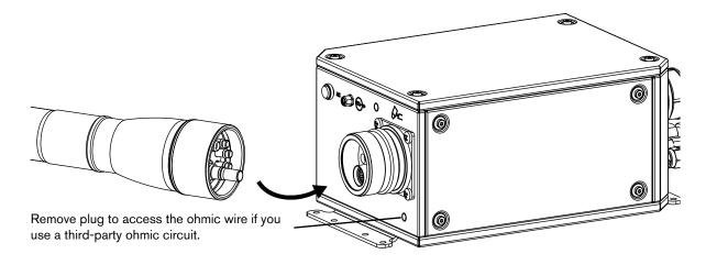
2. Connect the torch lead assembly to the TorchConnect console:
