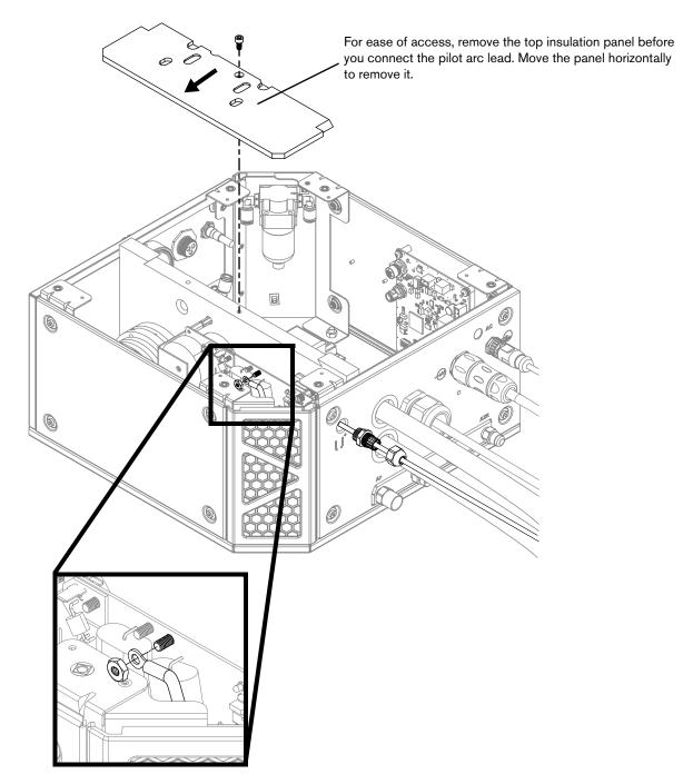
You do not need the strain relief nut. Remove the nut from the lead and tighten the strain relief into the panel on the gas connect console.
