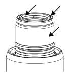
c. Apply a thin film of silicone lubricant (027055) to any O-ring that does not need replacement and that looks dry.
