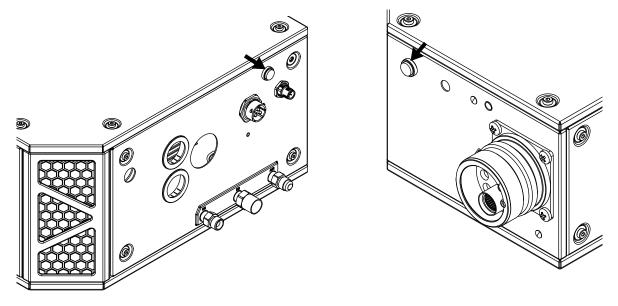
Figure 59 – Power-indicator LED on the gas connect console (left) and on the torch connect console (right)
