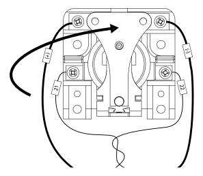
**6.** Measure the ohms between the nozzle and the workpiece. Less than 3 ohms is good. A value greater than 3 ohms indicates a faulty connection between the torch and ignition console, or between the ignition console and the power supply, or between the power supply work lead and workpiece.
