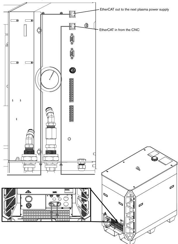
Figure 41 - Connect EtherCAT cables to plasma power supply
