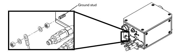
Found connection - Connect a ground lead (10 AWG) to the flat terminal on the torch mounting bracket
