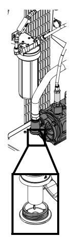
System components need the coolant to lubricate rotating surfaces. If air flows through the cutting system for longer than 30 seconds, it can eliminate the coolant necessary for lubrication.
