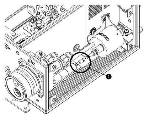
**4.** Use a digital multimeter to measure the resistance from the torch tip to the ohmic relay. Refer to Figure 68 on page 345.
