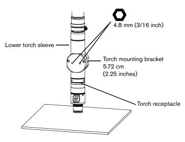
Figure 36 – Torch assembly in mounting bracket
