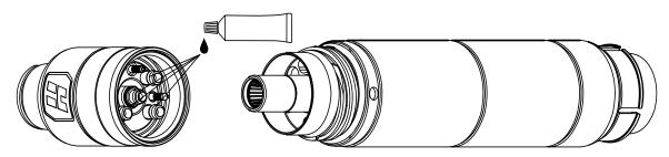
The O-rings should look shiny. Too much lubricant can prevent gas flow. Remove excess lubricant if found.
