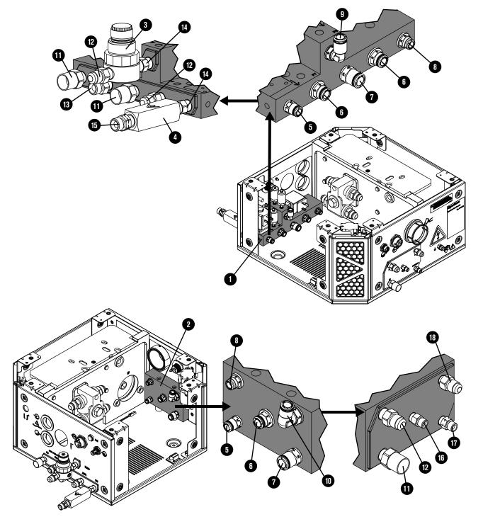
VWI gas connect console input and output manifolds and adapters
