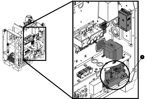
**3.** Install a temporary jumper wire between J5 (nozzle) **2** and J1 (work) **3** on the start circuit PCB 4 (141360).
