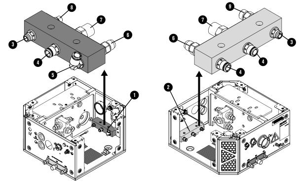
Core gas connect console manifolds and adapters
