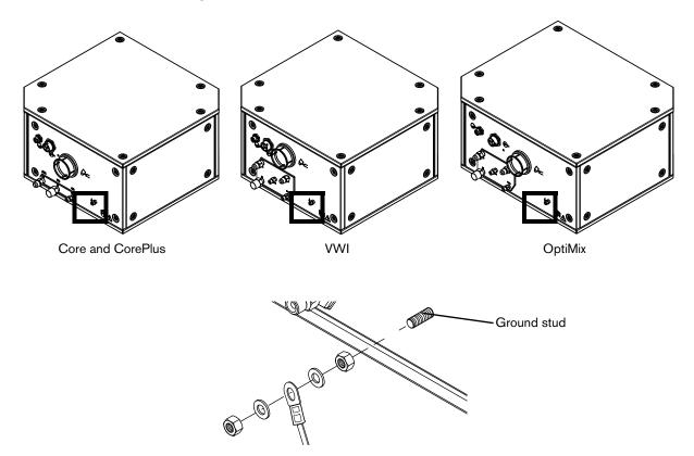
Figure 8 - TorchConnect console grounding (detail)
