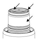
c. Use either 1 of the 2 available tools (104119 or 429013) to tighten the electrode. A tool is necessary to correctly install and tighten the electrode. Do not use your hands. If you fail to correctly install or tighten the electrode, torch damage can occur. Hypertherm recommends tightening the electrode to between 2.3 N·m − 2.8 N·m (20 in·lbf − 25 in·lbf) torque.
