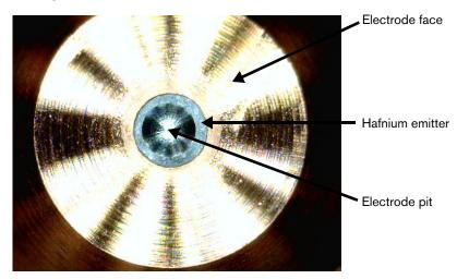
Figure 62 - Face of a new electrode (note hafnium emitter and electrode pit)
