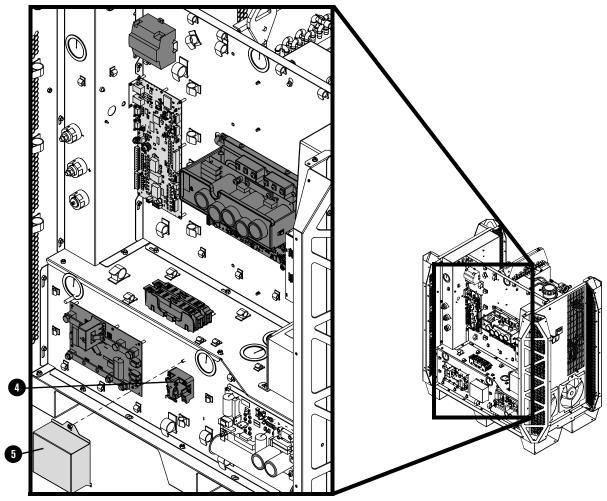
5. Have a second person close (push in) the contact on the pilot arc relay.
