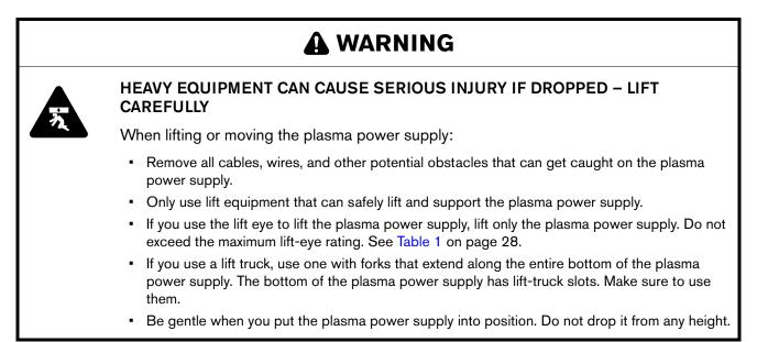
The XPR170 plasma power supply weighs 454.5 kg (1,002 lbs). You must use lift equipment to put it into position. Refer to Table 17. To protect the plasma power supply from drops and damage during lifting, make sure to balance it evenly and use slow speeds.
