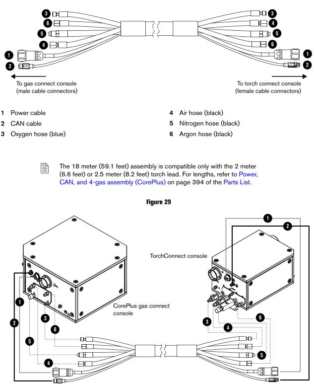
Figure 28 - Power cable, CAN cable, and 4-gas hose assembly
