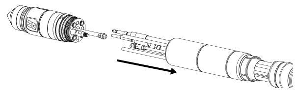
**4.** Align the color-coded leads in the torch lead assembly with the corresponding connectors in the torch receptacle.
