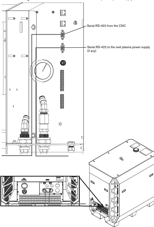
Figure 43 - Connect the serial RS-422 cable to the plasma power supply
