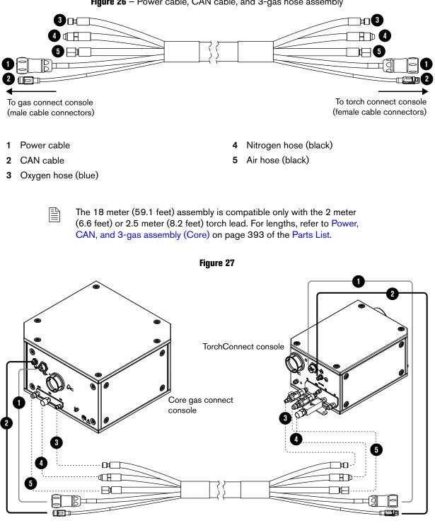
Figure 26 - Power cable, CAN cable, and 3-gas hose assembly
