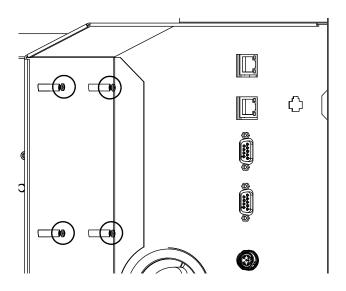
**3.** With J3 on top, use the 4 screws to install the board on the studs. Tighten the screws to 9.2 kg⋅cm (8.0 in⋅lb).
