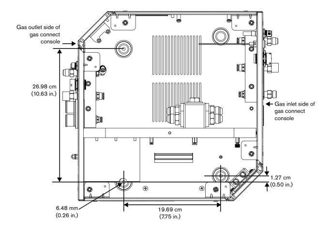
Figure 2 - Mounting dimensions for the OptiMix gas connect console
