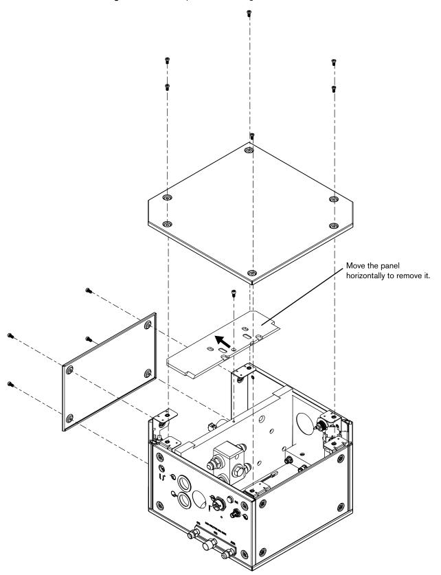
Figure 11 – Remove panels from the gas connect console
