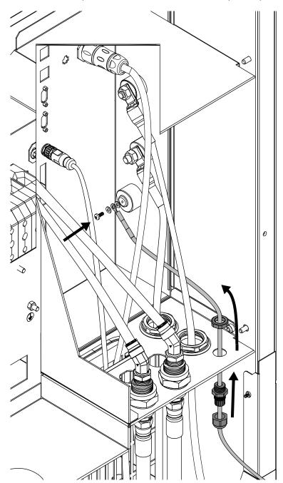
Figure 24 - Connect the pilot arc lead with strain relief to the gas connect console (Core, CorePlus, VWI, or OptiMix)
