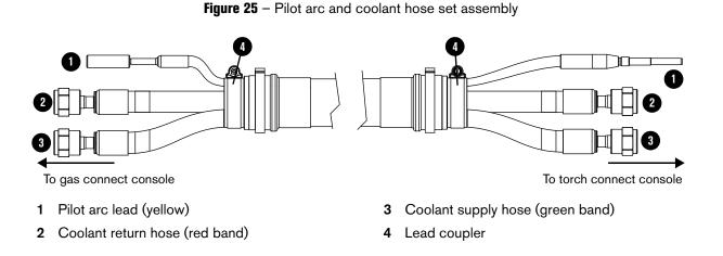
The 18 meter (59.1 feet) assembly is compatible only with the 2 meter (6.6 feet) or 2.5 meter (8.2 feet) torch lead. For lengths, refer to Pilot arc and coolant hose set assembly (Core or CorePlus) on page 393 of the Parts List.
