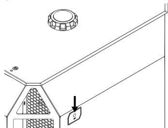
Figure 58 - Power-indicator LED on the plasma power supply
