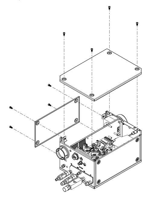
Figure 12 - Remove top and side panels from the TorchConnect console
