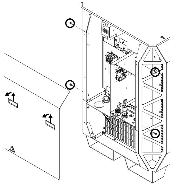
For installation usually it is necessary to remove only the rear panel.
