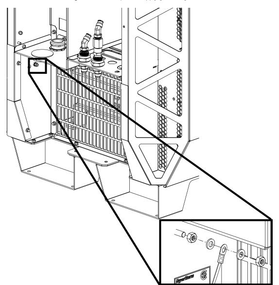
Figure 6 - Plasma power supply grounding (detail)
