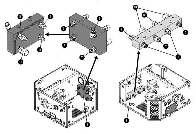
CorePlus gas connect console manifolds and adapters
