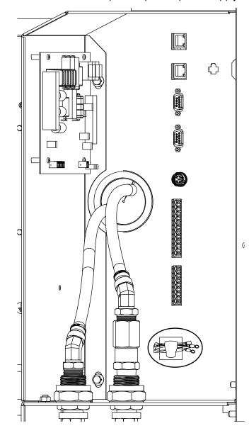
1. Remove the wire bundle from the wire clip in the plasma power supply.
