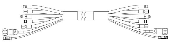
The 18 meter (59.1 feet) assembly is compatible only with the 2 meter (6.6 feet) or 2.5 meter (8.2 feet) torch lead.
