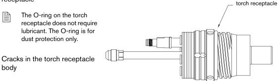
3. Replace the O-ring if it has damage or excess wear.
