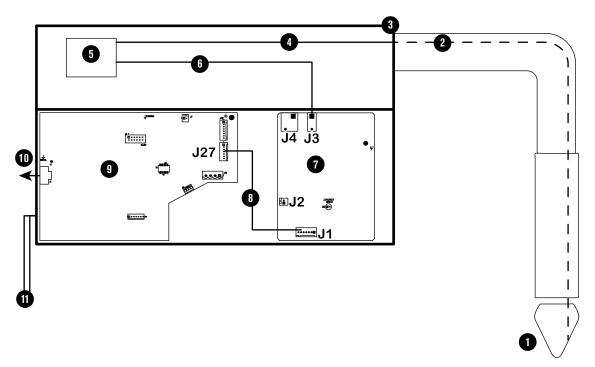
Figure 55 - Internal ohmic diagram
