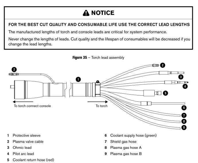
The 6 meter (20 feet) lead is compatible only with gas assemblies that are 7.5 meters (24.6 feet) or less. For lengths, refer to Torch lead on page 397 of the Parts List.
