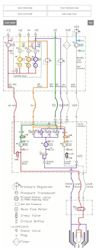
Figure 54 - Example diagram-view screen that shows the gas system status
