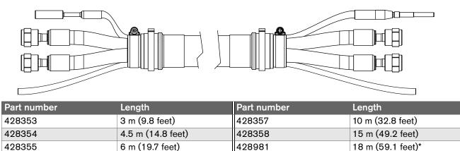
\* The 18 meter (59.1 feet) assembly is compatible only with the 2 meter (6.6 feet) or 2.5 meter (8.2 feet) torch lead.
