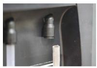
3. Use the tube cleaning brush to clean the inner surfaces of the tube.
