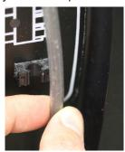
**2.** Disconnect the tube from the push-to-connect fitting on top of the SMI by pushing up on the collar of the fitting while pulling down on the tube.
