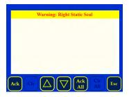
Touch **Ack** (acknowledge) or **Ack All** (acknowledge all) on the screen. The beacon light stops flashing and the alarm screen closes.
